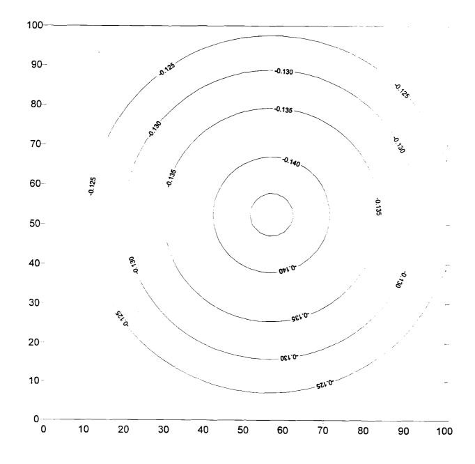
Figure 5-9 AIR3D Modeling Results: Pressure Distribution
