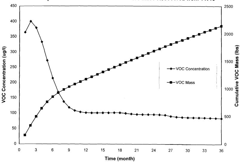
Figure 5-27 VT3D Modeling Results for Case 4 VOC Vapor Concentrations and Cumulative Mass Recovered from VW14
