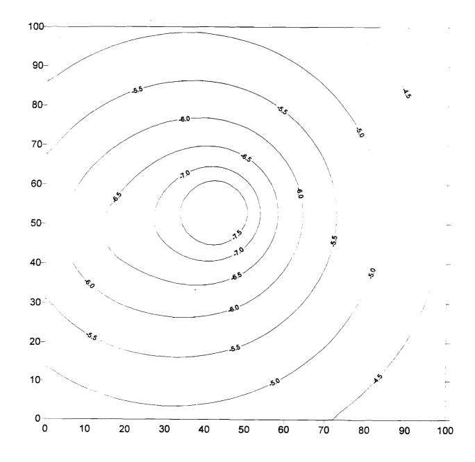
Figure 5-23 AIR3D Modeling Results: Pressure Distribution
