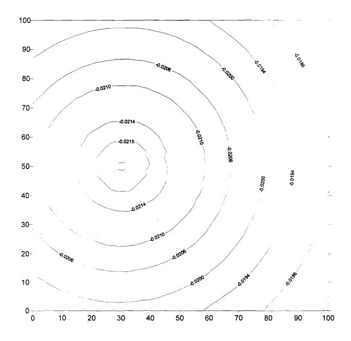
Figure 5-15 AIR3D Modeling Results: Pressure Distribution
