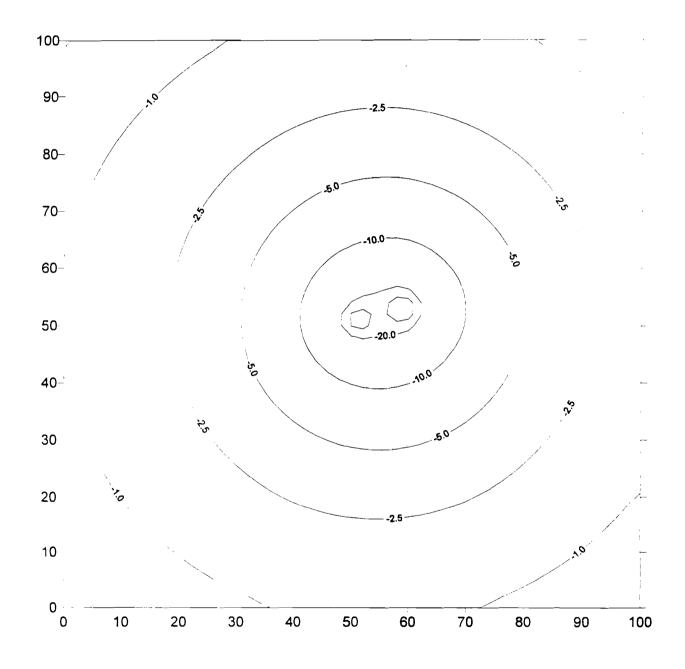
Figure 5-7 AIR3D Modeling Results: Pressure Distribution
