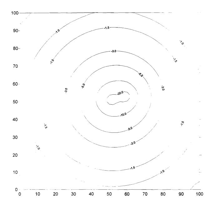
Figure 5-6 AIR3D Modeling Results: Pressure Distribution
