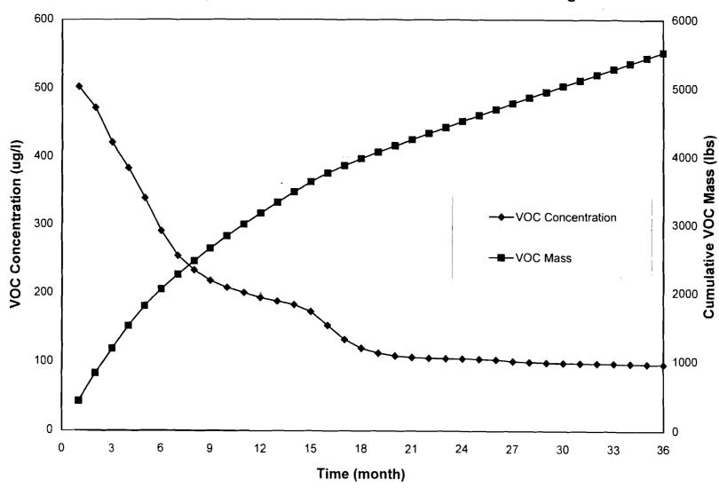
Figure 5-28b VT3D Modeling Results for Case 4 Cumulative Recovery of 93% of Total VOC Mass
