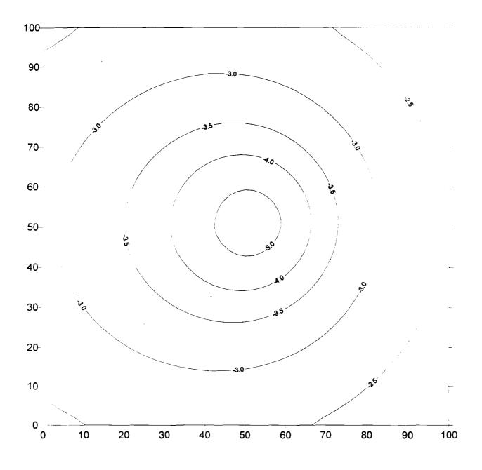
Figure 5-22 AIR3D Modeling Results: Pressure Distribution
