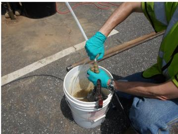
All groundwater samples were shipped to TAL, under proper Chain of Custody procedures. All groundwater samples were analyzed for VOCs by USEPA Method 8260.
