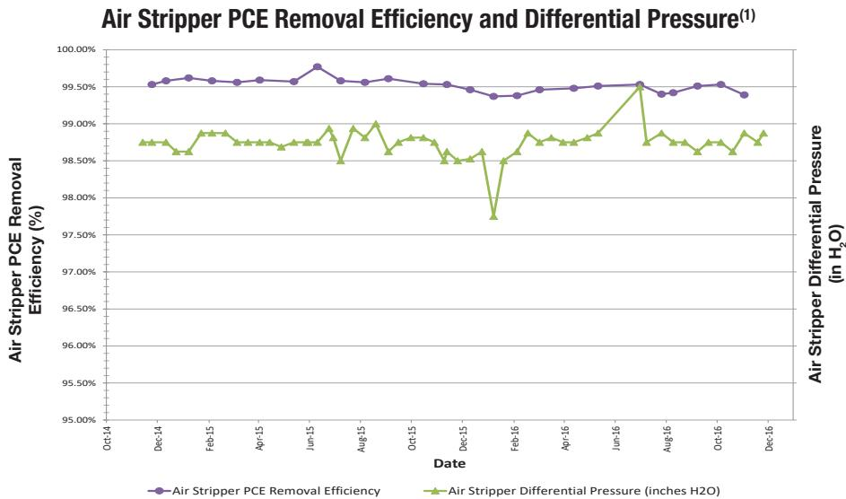
1. The approximate PCE removal efficiency for the low-profile stacked-tray air stripper ranged from 99.35% to 99.51% during this reporting period. Additionally, the average differential pressure across the low-profile air stripper was well below 45 inches of water (manufacturer's recommended threshold for equipment maintenance) during this reporting period.
