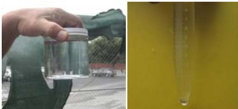
Photographs 3-3 and 3-4: EW-1I sand content sample (left) and 0.05 mg/L of sand deposited into vial (right).
