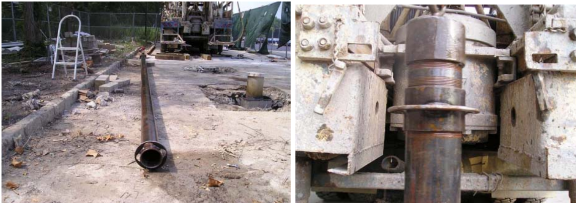
Photographs 3-1 and 3-2: Plumbness and alignment testing device, total length view (left) and top view (right).
