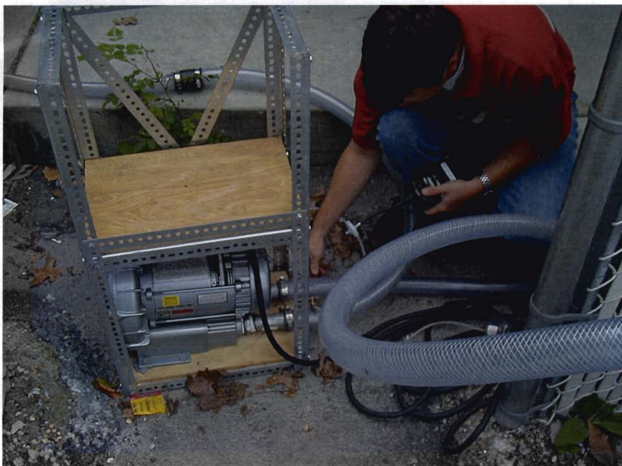
Portable 1 H.P. blower used to test SVE wells at 45 Sea Cliff Avenue site.
