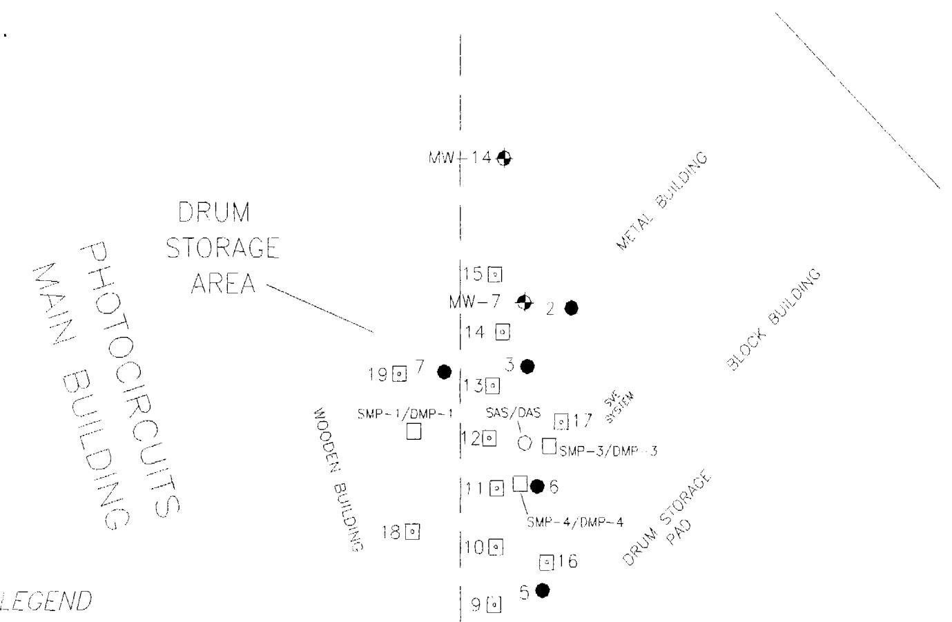
Figure 2. Site Map Showing Injection Points and Monitoring Wells Within Pilot Cell
