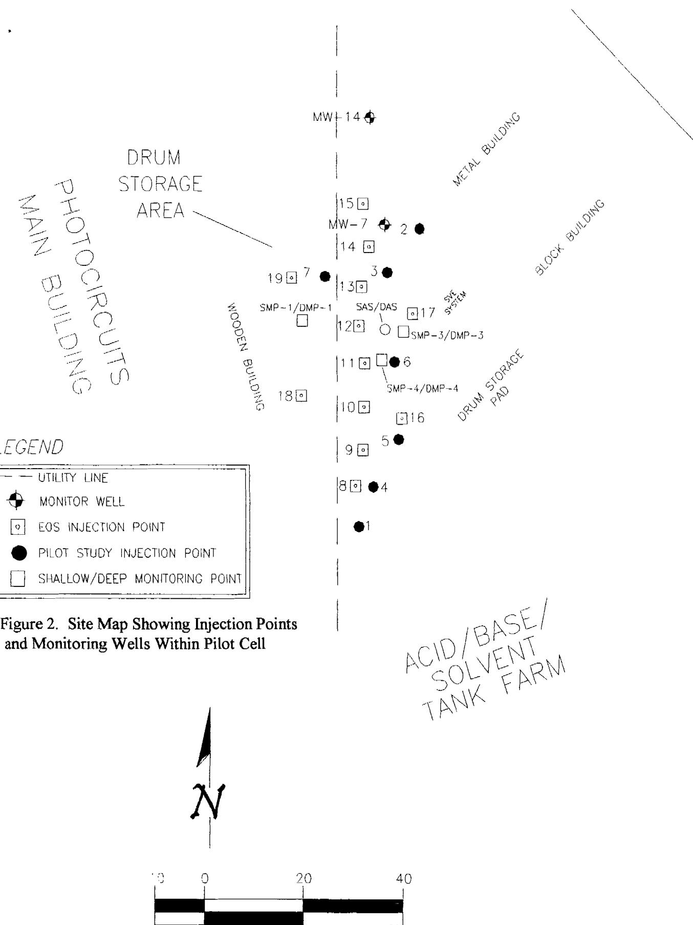
Figure 2. Site Map Showing Injection Points and Monitoring Wells Within Pilot Cell
