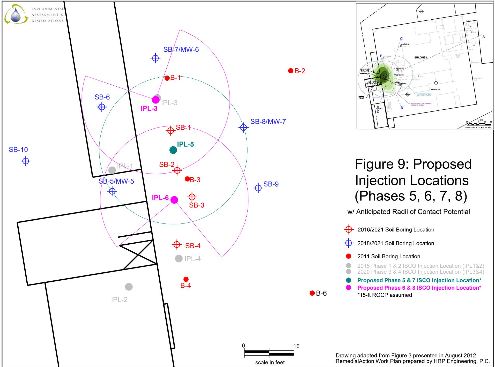
Drawing adapted from Figure 3 presented in August 2012 RemedialAction Work Plan prepared by HRP Engineering, P.C.
