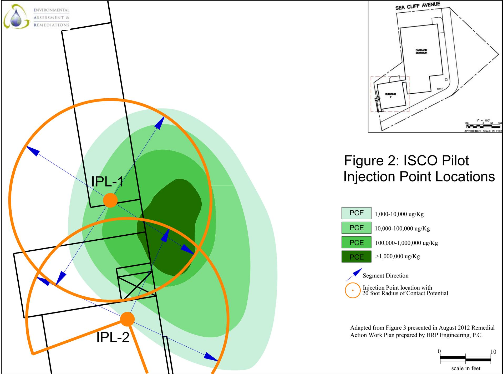
Figure 2: ISCO Pilot Injection Point Locations
