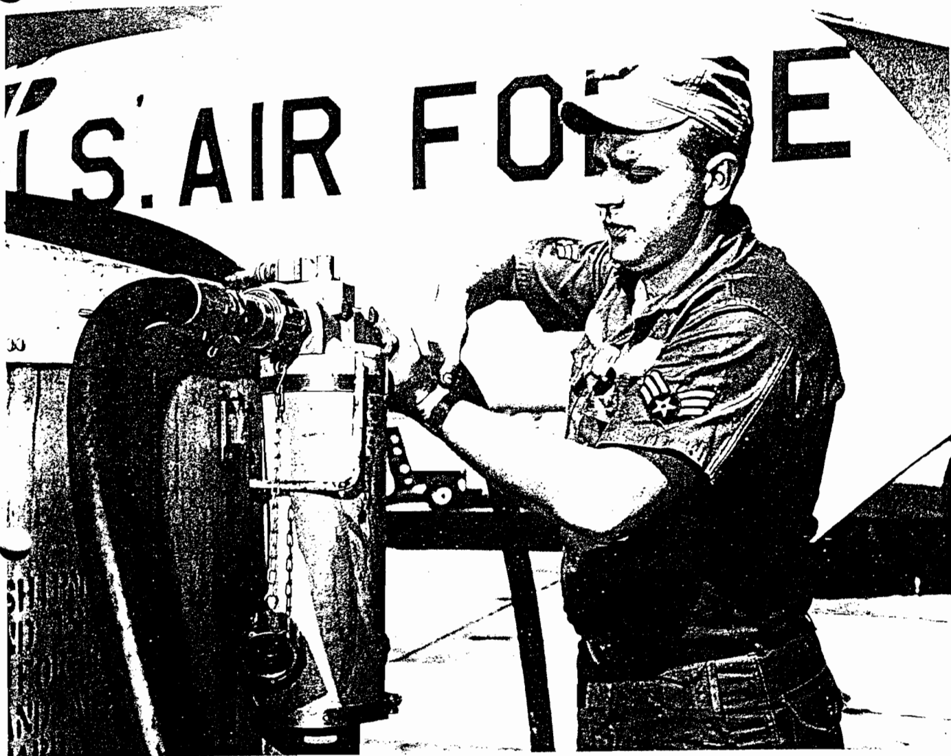
Air Force technician connects ULTIPOR 9 TRIPHANI filter, now standard equipment on Air Force hydraulic ground service units.
