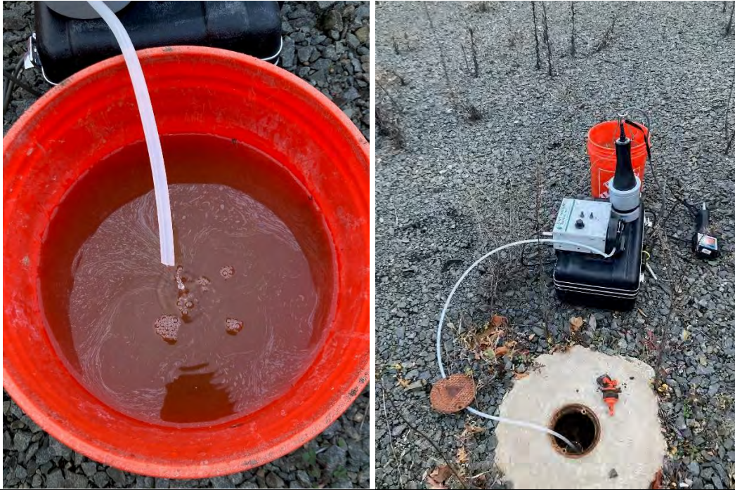
Sheen observed from MW-8 (left), Setup on MW-8
