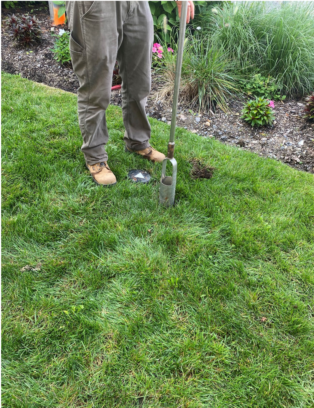
Figure 1: installing new temporary soil vapor point near VMP-5
