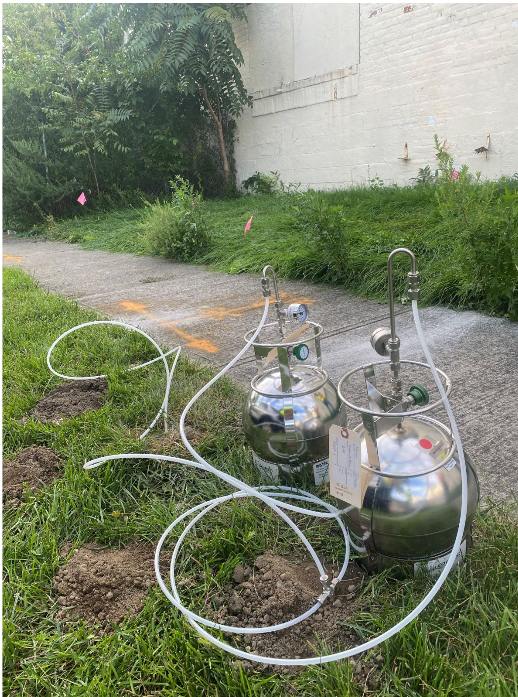
Figure 1: Collecting soil vapor and a duplicate at the temporary soil vapor point location near VMP-4. Facing south southeast
