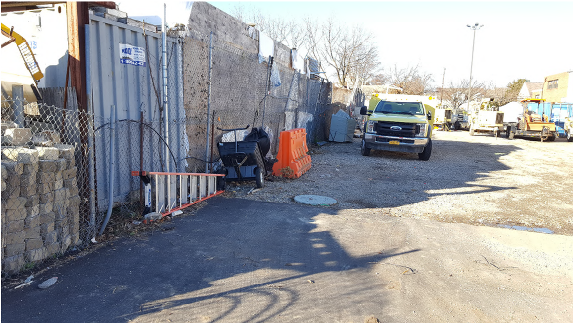
Photograph #9 – View of yard looking north along west property line. Protective concrete disc covering well vault for monitoring well MW-5.
