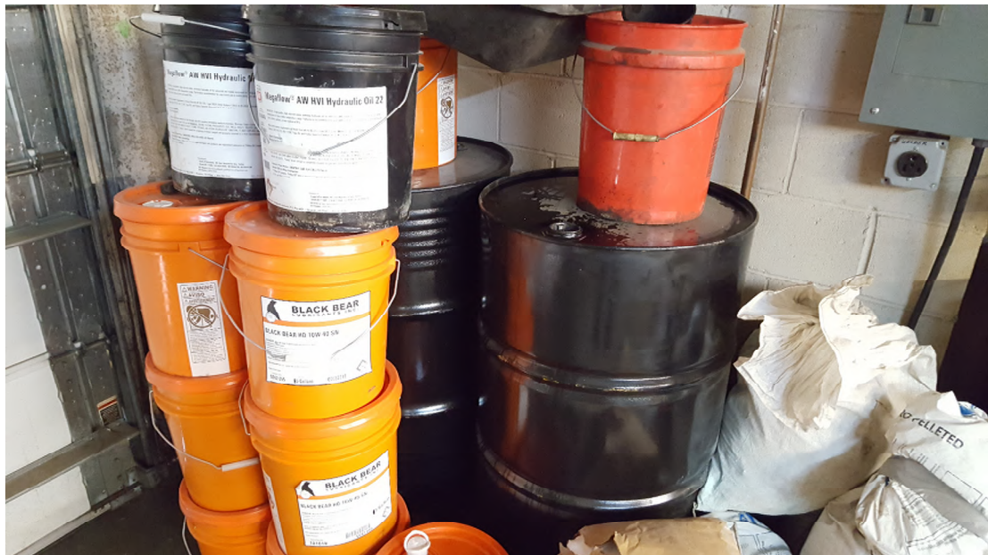
Photograph #8 - Ground floor interior of office/garage building, southwest corner. 5-gallon containers of motor oil and hydraulic fluid. Two 55-gallon drums for used oil, collected by permitted recycler.
