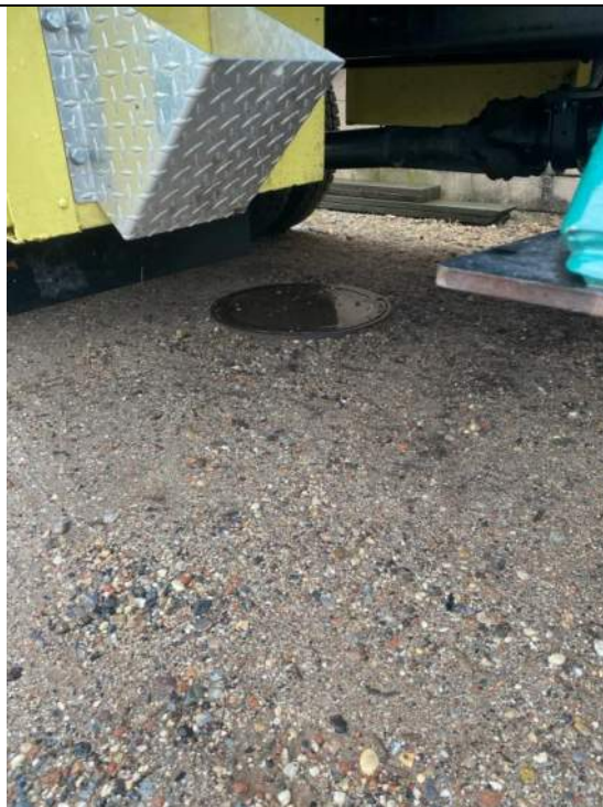
Photograph #12 – View of yard looking east along east property line. Protective metal manhole covering well vault for monitoring well MW-3.
