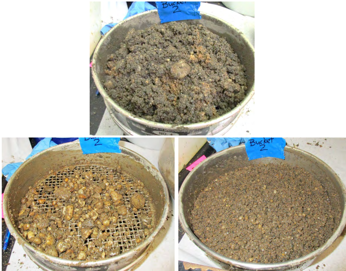
Figure 2. Bucket 2 Soil As Received (top), +4 Mesh (bottom left) and -4 Mesh (bottom right).
