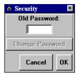
3. You will then be prompted to enter the **New Password** in the text box. Recall that the password can be up to three characters consisting of the numbers 0-9 and the letters A-Z. After clicking on the **OK** button or hitting the enter key, you will be prompted for the new password again.
