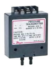
The Dwyer Series 616 Differential Pressure Transmitter senses the pressure of air and compatible gases and sends a standard 4-20 mA output signal. A wide range of models are available factory calibrated to specific ranges as listed in the chart below. The span and zero controls are for use when checking calibration. They are not intended for re-ranging to a significantly different span. Versatile circuit design enables operation in 2, 3 or 4-wire current loops.
