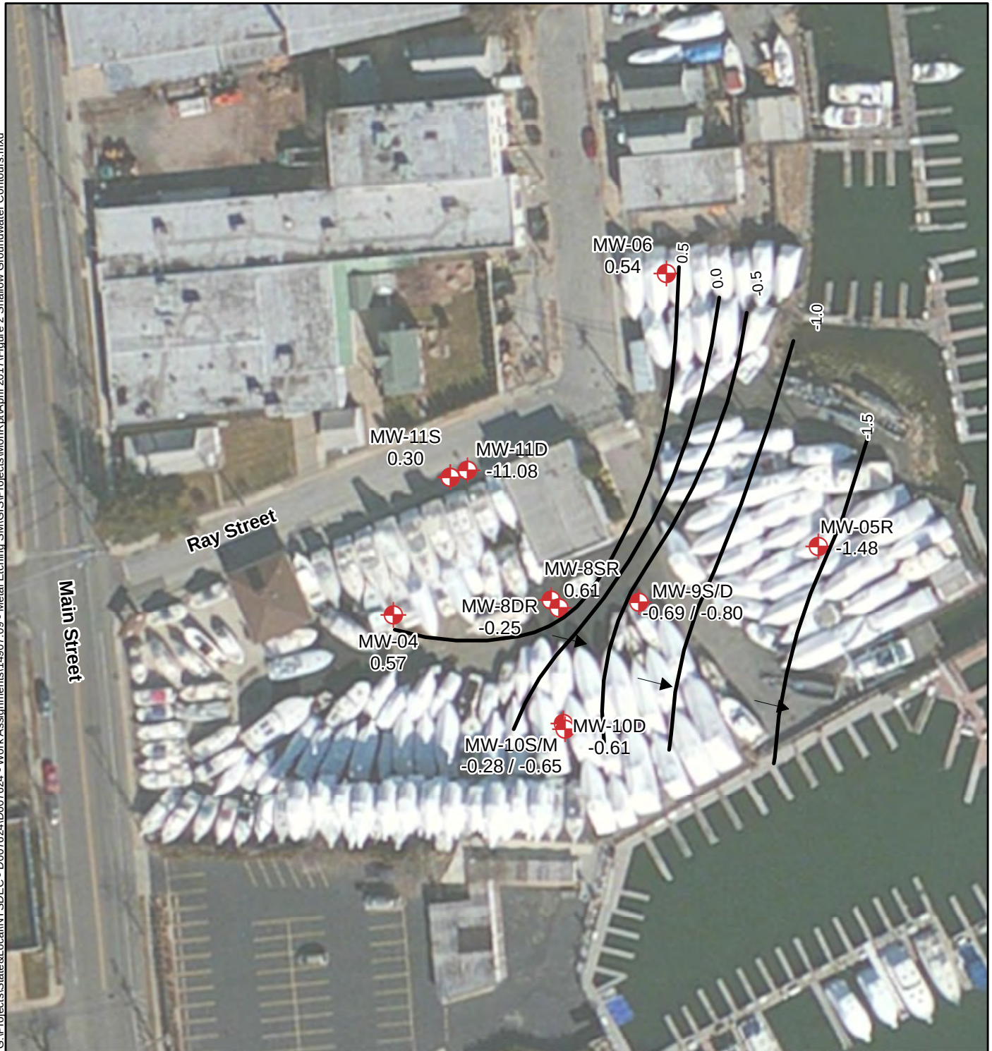
Figure 2 Shallow Groundwater Contours Low Tide Conditions April 2017 Metal Etching Site (130110) Freeport, New York
