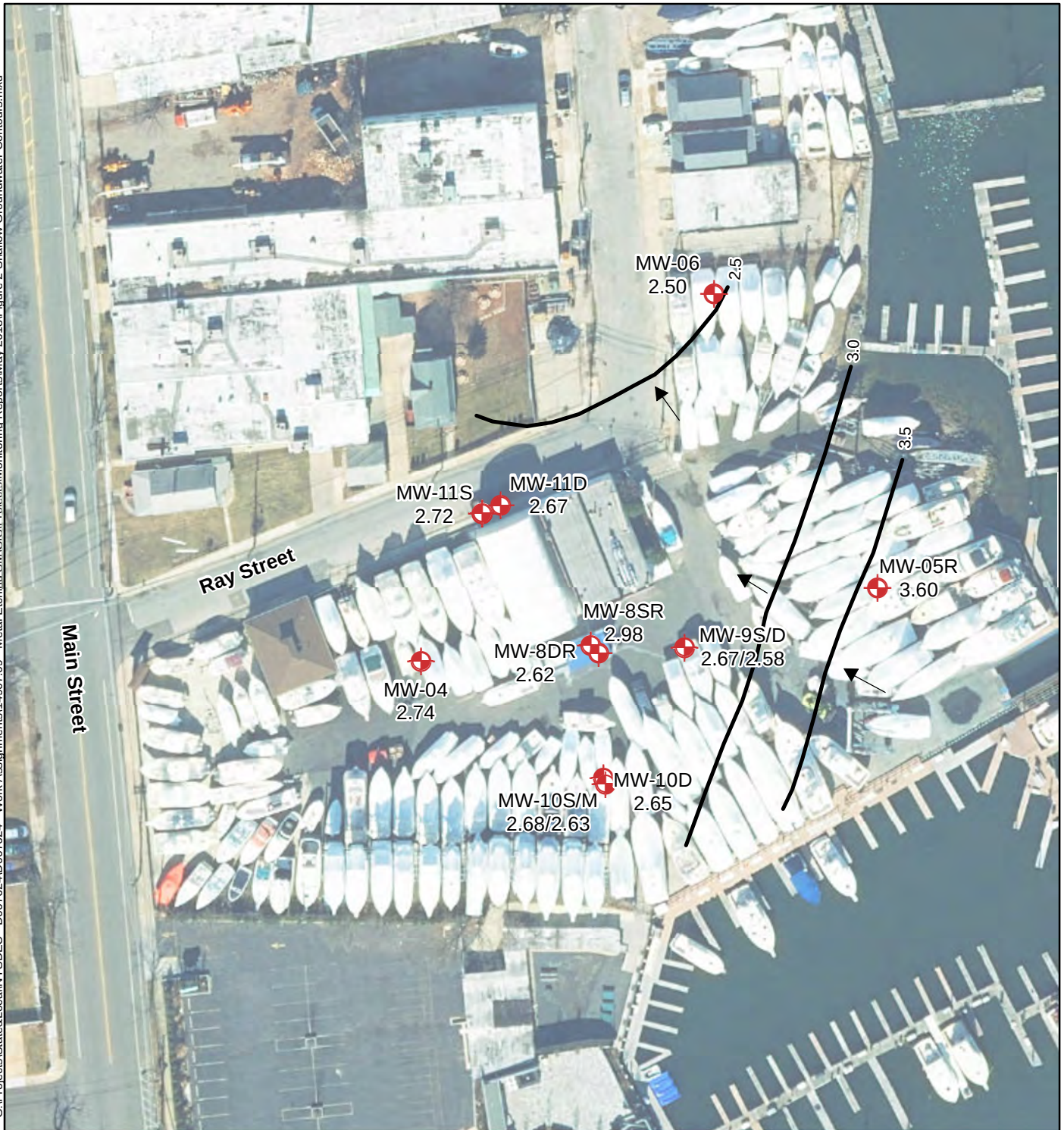
Figure 2 Shallow Groundwater Contours High-Tide Conditions March 2018 Metal Etching Site (130110) Freeport, New York
