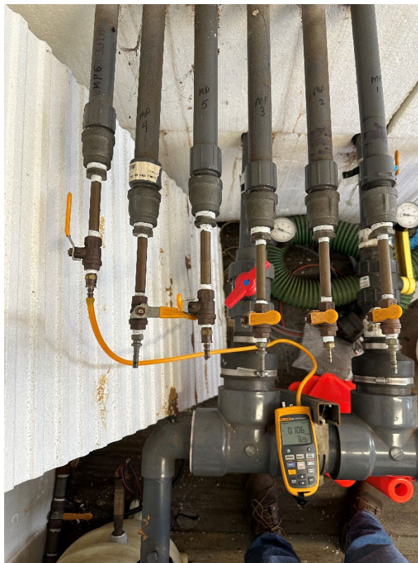
Photograph 4: View of the vacuum measurement from MP-6.
