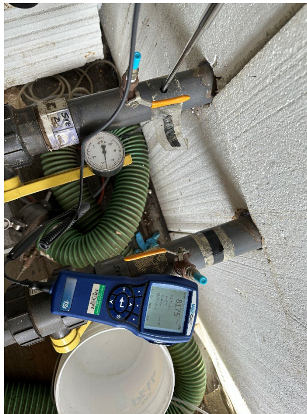
Photograph 4: View of the velocity measurement from SVE-2.
