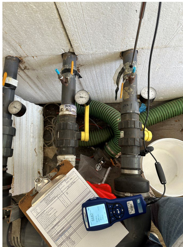
Photograph 4: View of the velocity measurement from SVE-1.
