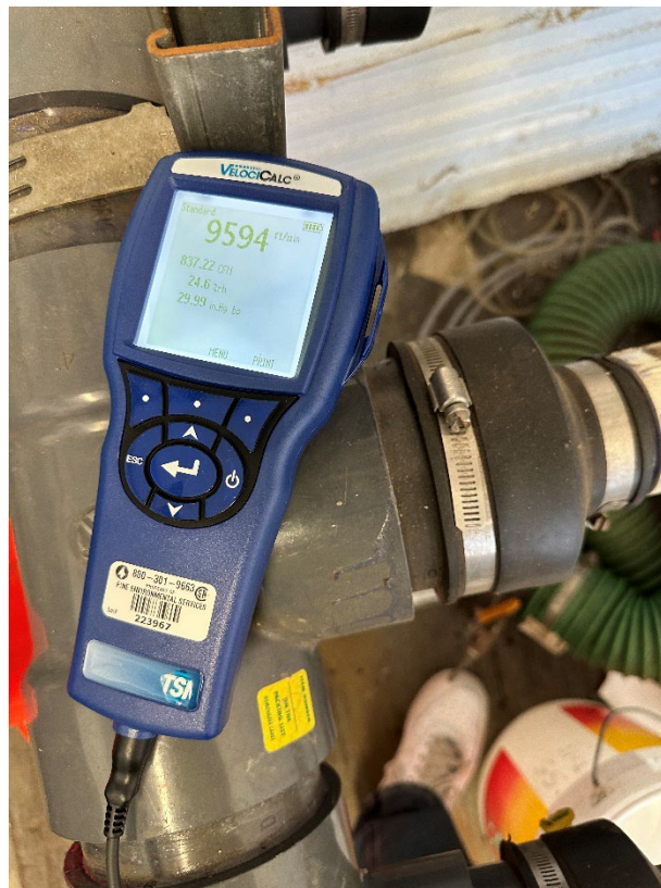
Photograph 4: View of the velocity measurement from SVE-2.
