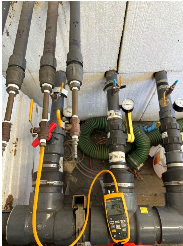
Photograph 3: View of the vacuum measurement from MP-2.
