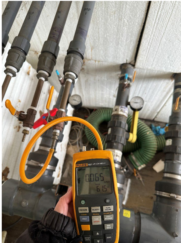
Photograph 3: View of the vacuum measurement from MP-1.
