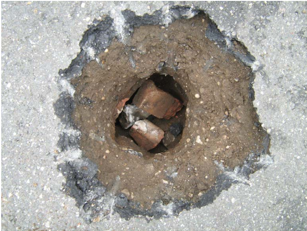
Photo 6: Bricks and concrete fragments in canceled soil boring location EGCSB-06
