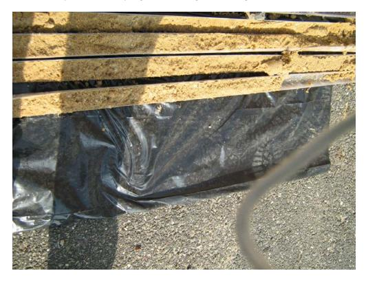
Photo 8: Geoprobe soil core showing non-impacted soil
