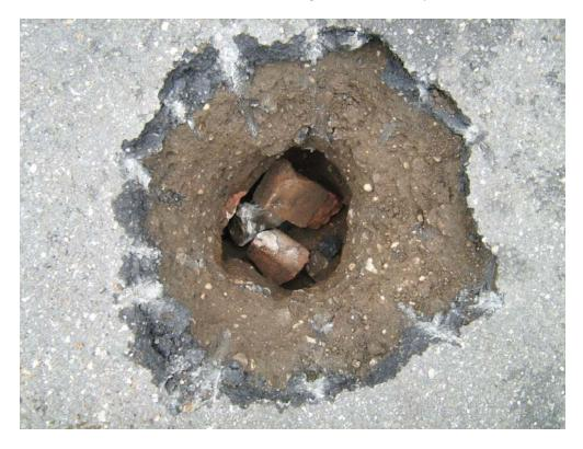
Photo 6: Bricks and concrete fragments in canceled soil boring location EGCSB-06
