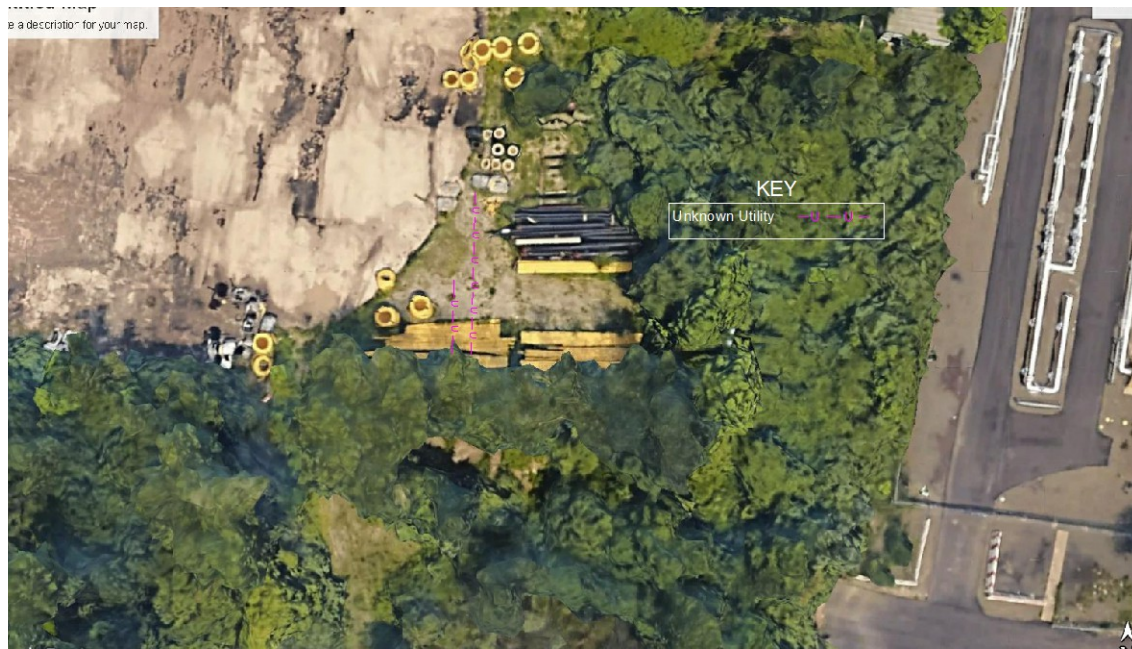
Figure 4: Confirmed utilities. Running from south to north the larger diameter pipe is located on the left side while the smaller pipe at approximately 1ft is located on the right. *(Not to scale)
