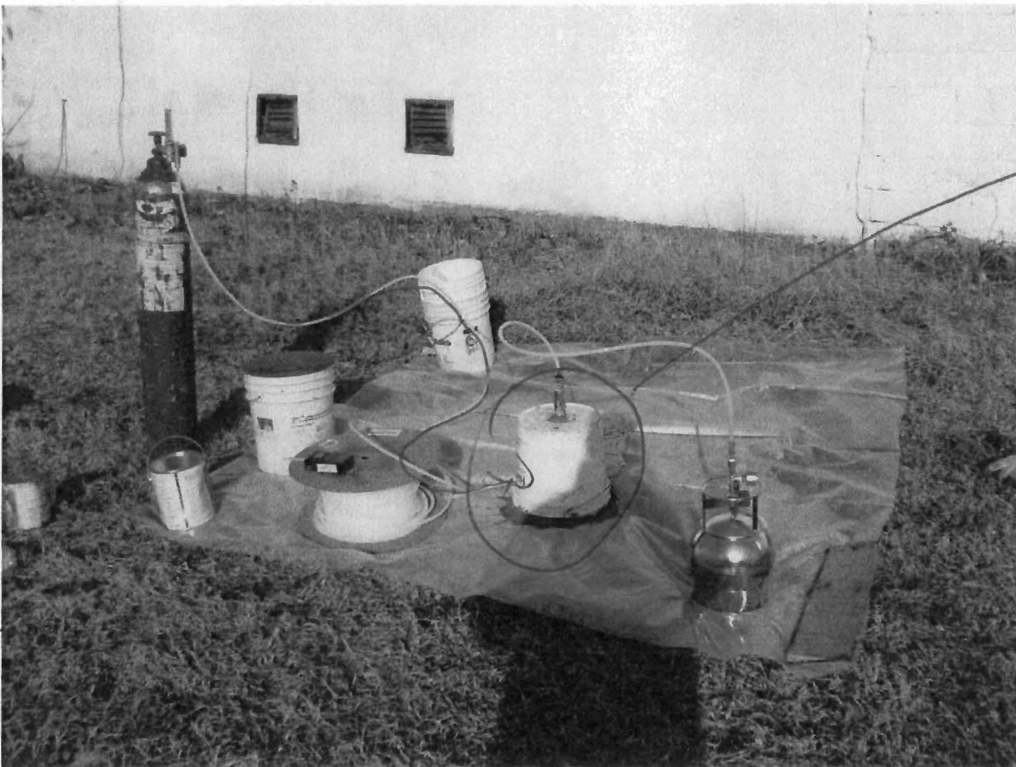
Photograph No. 2: Soil gas sampling set-up.
