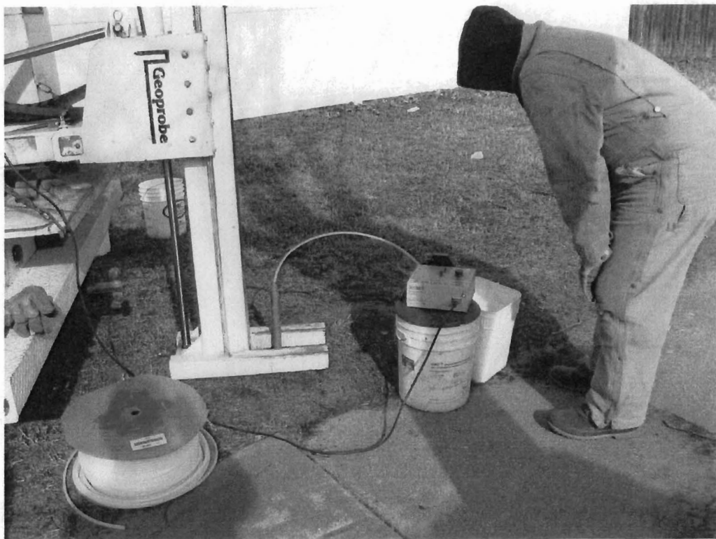
Photograph No. 4: Groundwater sampling.
