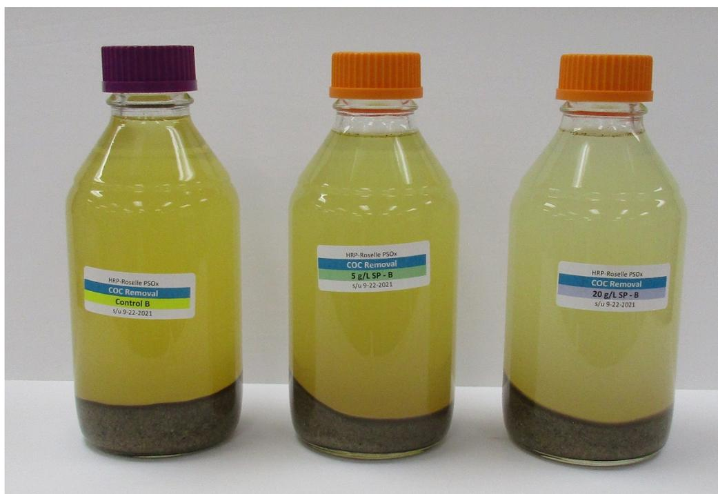
**Figure 1. COC Removal Reactors at Day 28 – Initial Tests.** From left: Control, PersulfOx<sup>®</sup> Low, PersulfOx<sup>®</sup> High.
