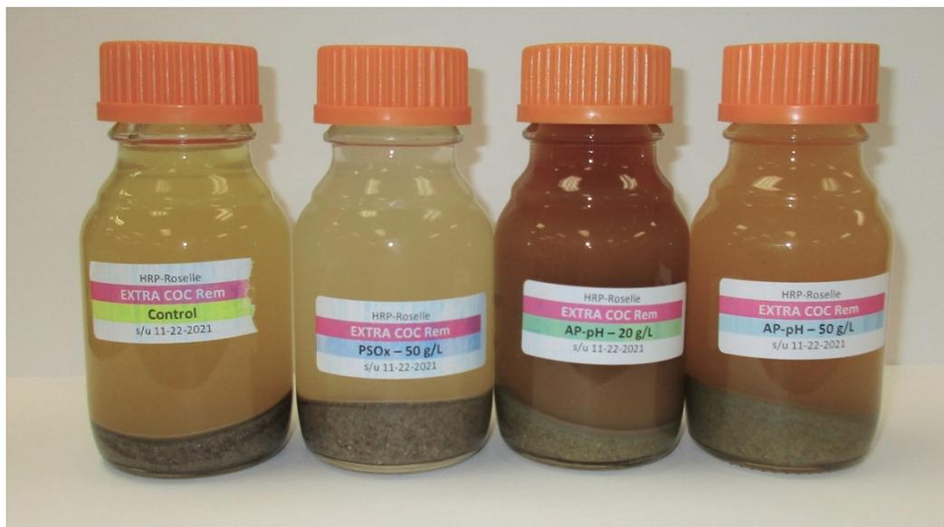
**Figure 2. COC Removal Reactors at Day 28 – *Follow-up Tests.*** From left: Control, PersulfOx<sup>®</sup> 50 g/L, AP-pH-20 g/L, AP-pH-50 g/L.
