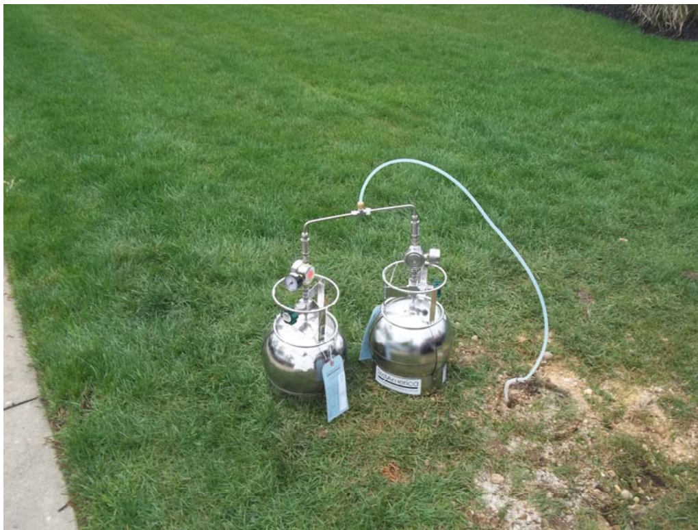
Soil Vapor Sampling – Sulzer Metco, Inc. Split Sample Collected with Tee
