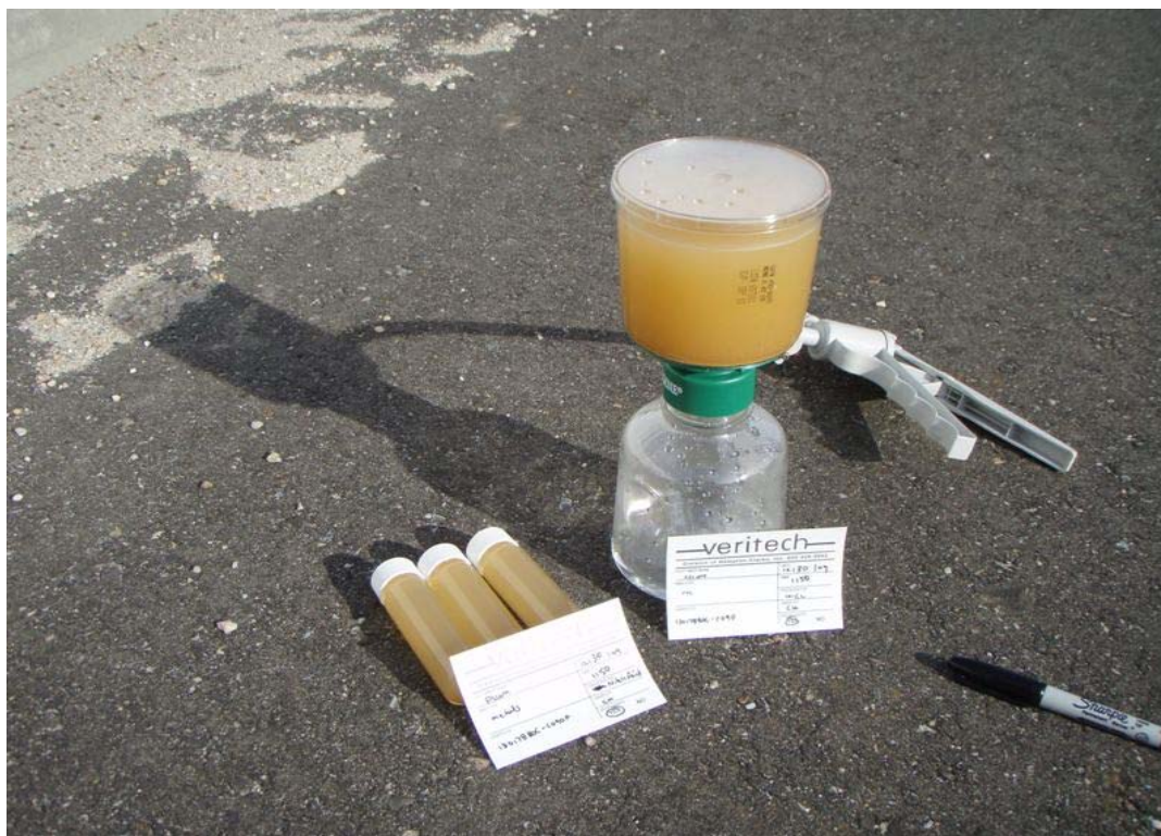
VOC Samples and Field Filtering for Metals Analysis
