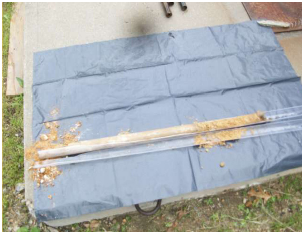
Soil Boring Samples Collected in Macrocores (SB-5. 5 ft to 10 ft shown)
