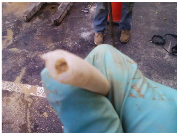
Sand clogging sample tubing
