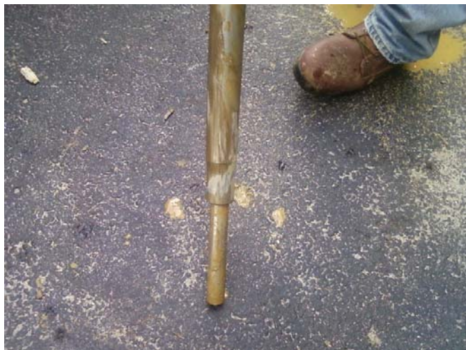
Sand jamming hydropunch rod/screen
