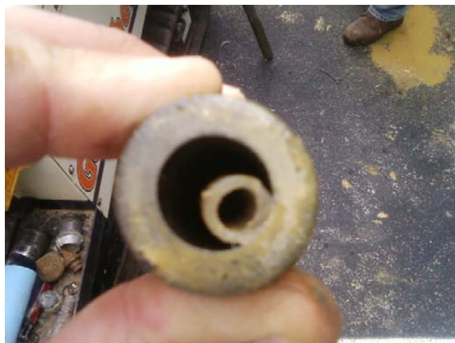
Sand and tubing stuck within drive rod
