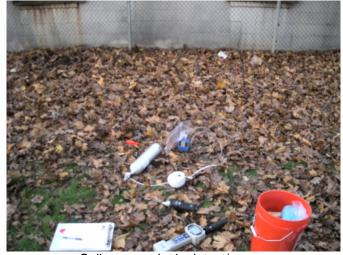
Soil vapor point leak test/purge
