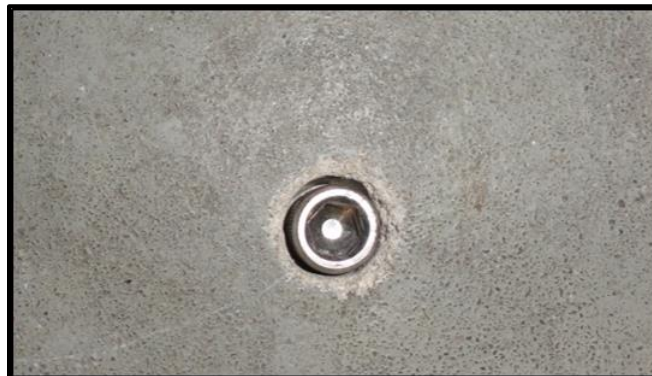
Permanent Sub Slab Test Port
