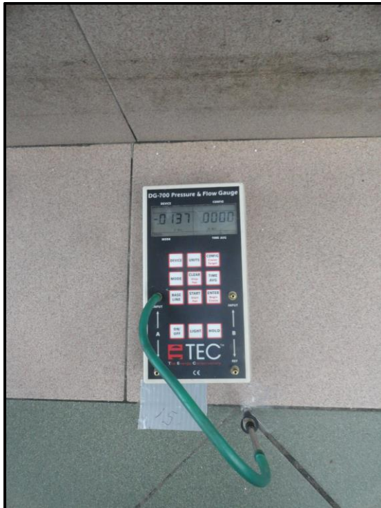
Measuring Sub Slab Differential Pressures at Remote Test Holes
