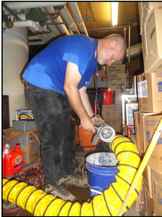
Measuring Airflow Yields at Known Amounts of Applied Vacuum
