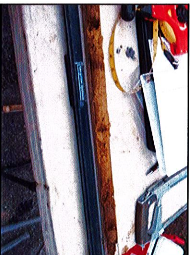
Photograph No. 4 – Medium to coarse sand and gravel encountered within soil borings exterior to the building.
