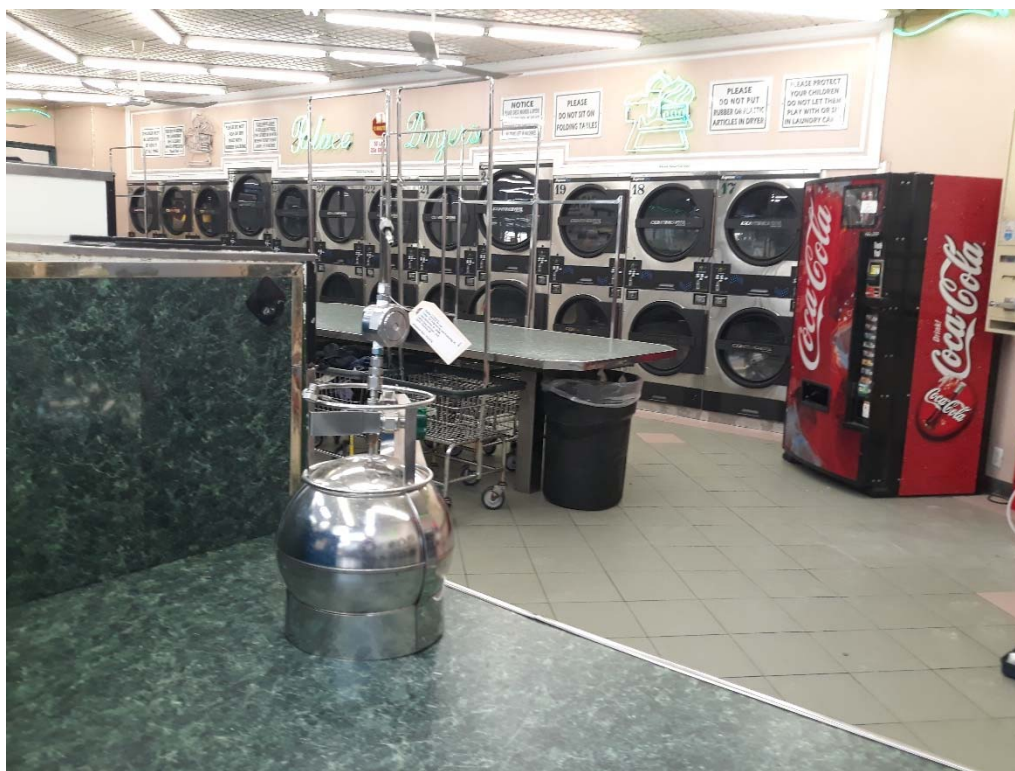
Photo 2 Co-located indoor air sampling canister in Unit 179A.
