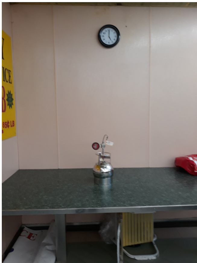
Photo 4- Co-located indoor air sample in Unit 181A.
