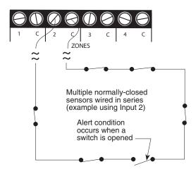
Figure 2-8. Multiple Normally Closed Sensors
