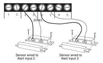
Figure 2-7 Two Sensors Wired to Adjacent Zones
