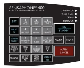
Figure 3-1. The Model 400 Keypad
