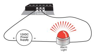
Figure 1: Relay output connected to alarm
