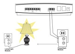
Figure 2: X10 Lighting Control Setup
