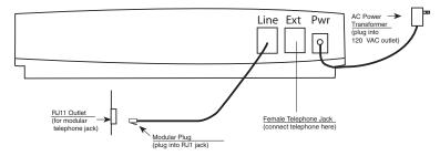
Figure 2-4. Installing the Telephone Line
