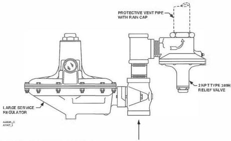
Figure 4. Typical Installation of a 289 Series Relief Valve
