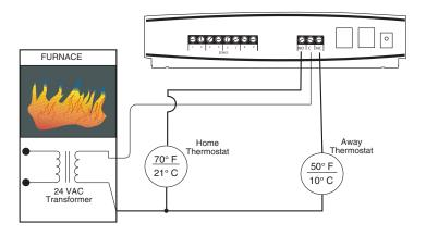
Figure 1: Dual Thermostat Setup
