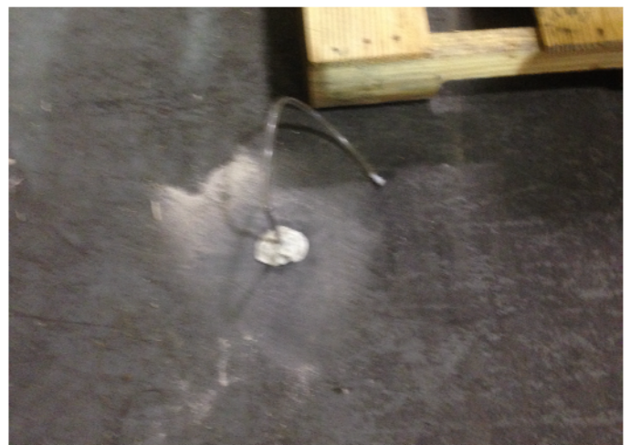
View of temporary differential point during the pilot test.
