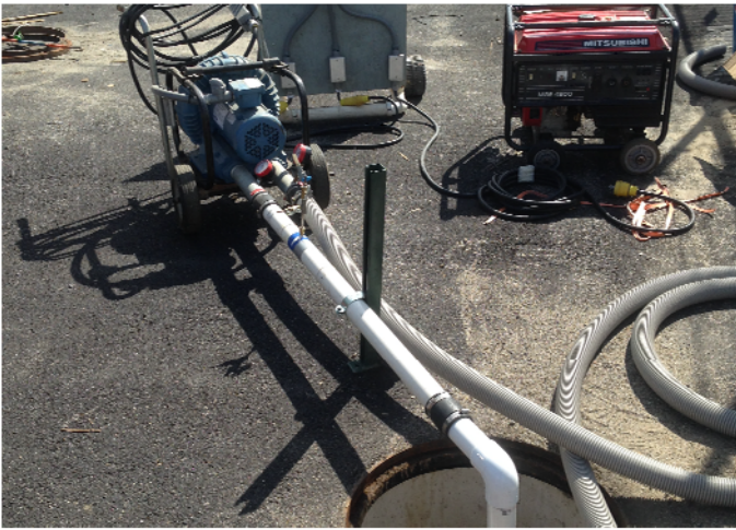
View of blower attached to exterior SVE well (SVE-2) during pilot test.
