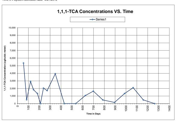
System Analytical Data for Treated Air in ug/cubic meter
