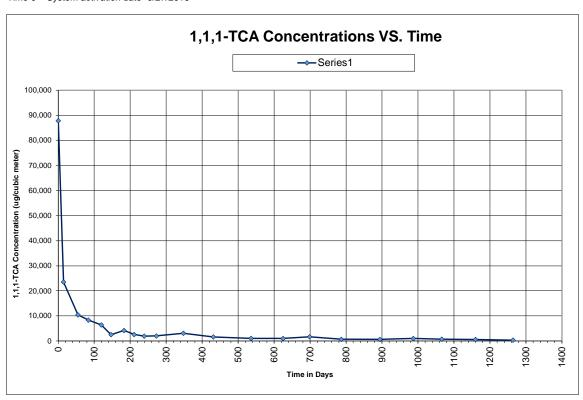
System Analytic Data for Mid Carbon Samples in ug/cubic meter
