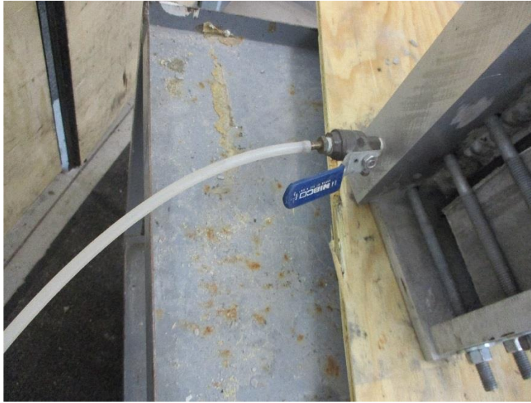
Typical loaded specimen – filling chamber with water
