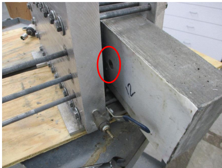
Typical loading of the specimen into the apparatus Note: the "rupture" is exposed to the water in the chamber
