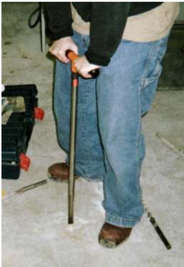
Sub-Slab Soil Sampling Equipment
