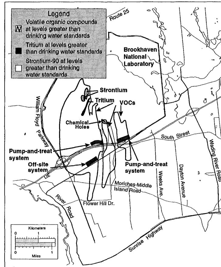
This figure shows the locations of the Operable Unit III groundwater contaminants, and VOC treatment systems. The Chemical Holes are a source of both VOCs and strontium-90.
