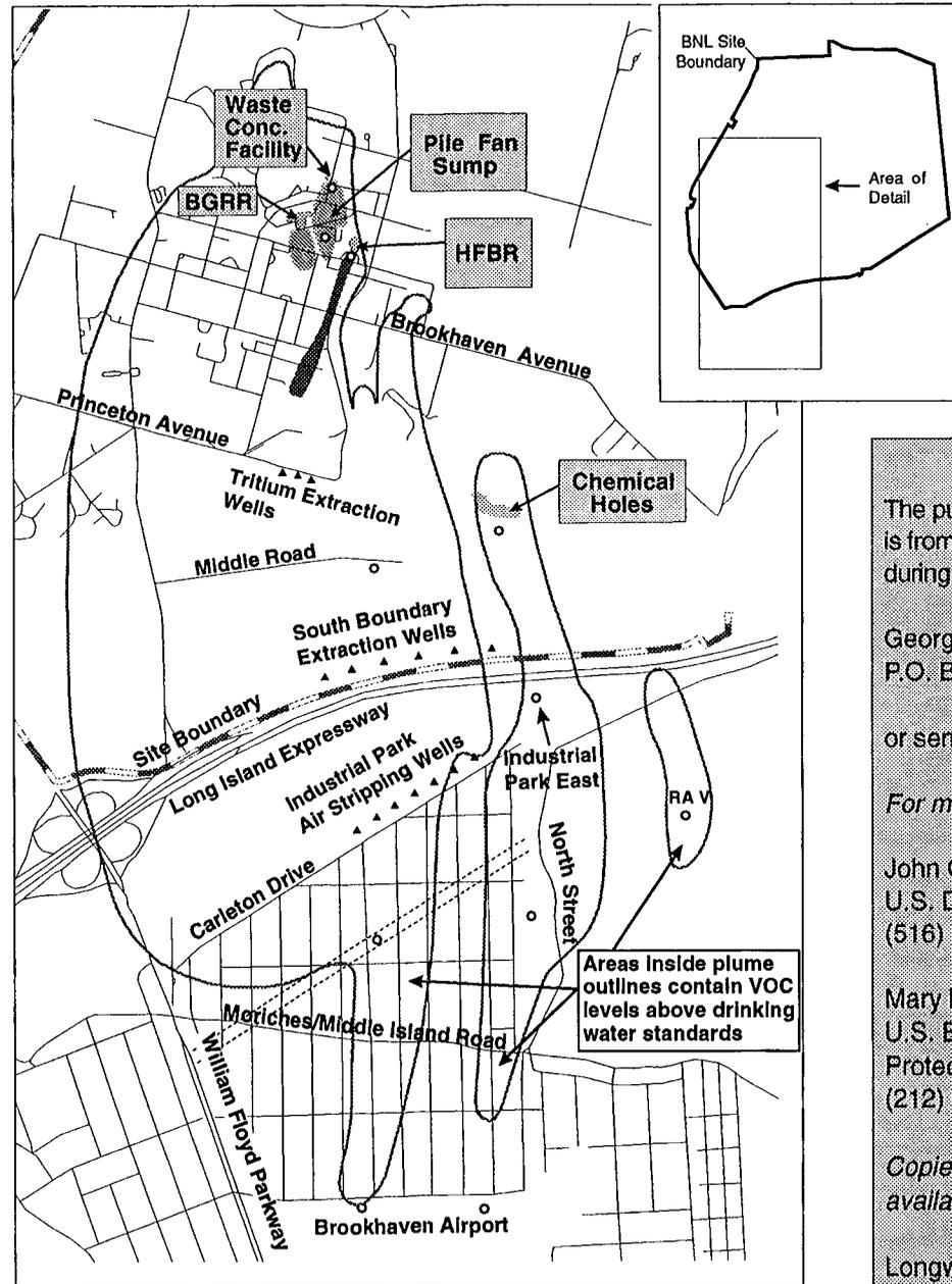
This figure shows the locations of groundwater contaminants at levels above drinking water standards as well as the locations of the tritium and strontium-90 sources. It also indicates proposed locations for treatment systems.
