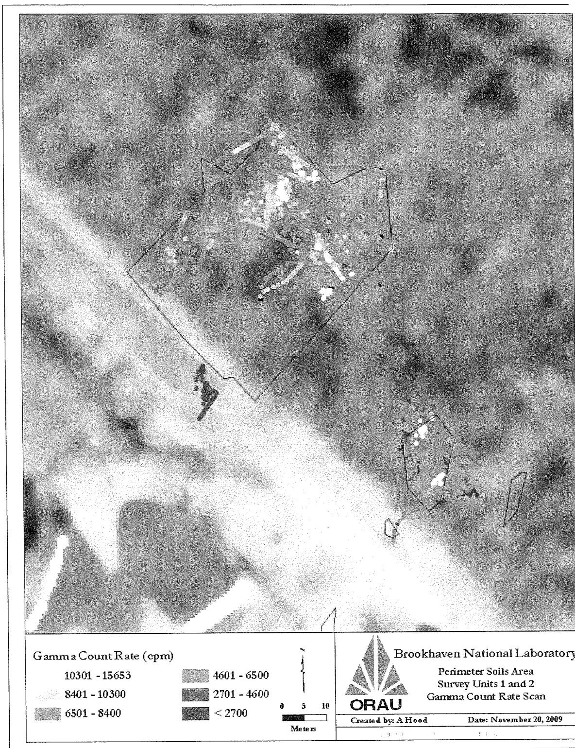
Figure A-3. Perimeter Soils Area Gamma Count Rate Scan Survey Units 1 and 2
