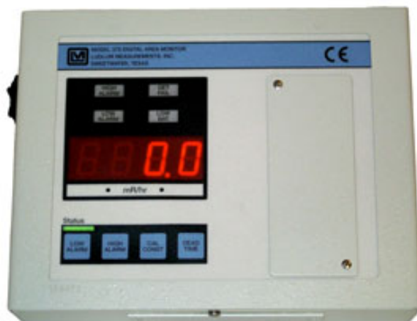
Figure 3-6. Radiation Detection and Alarm System (RDAS) instrument Ludlum 375/4.
