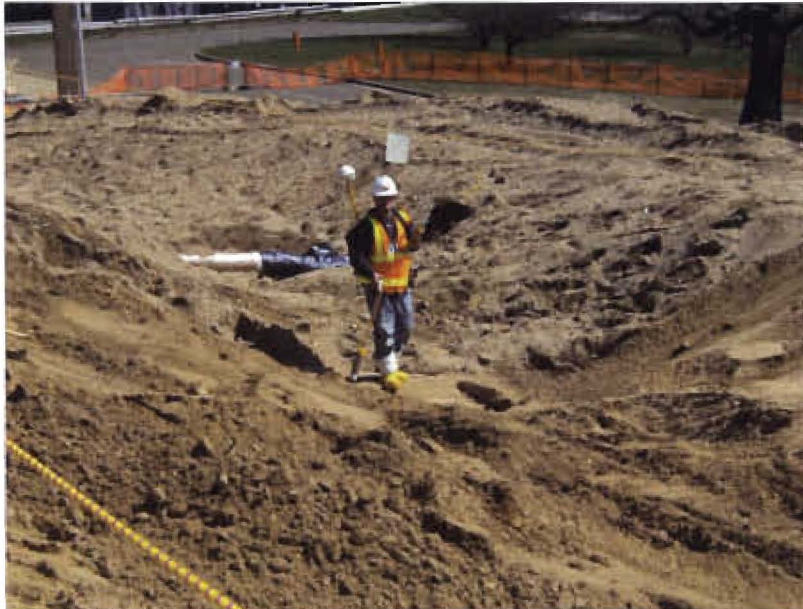
Photograph 5 – Performing radiological walkover survey of trench during Phase I
