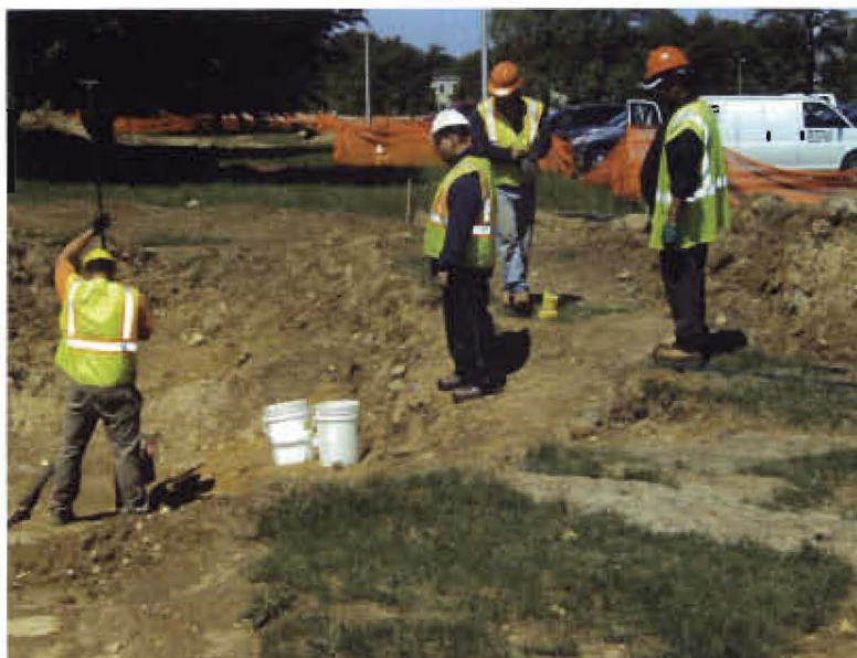
Photograph 6 – Collection of FSS core samples during Phase II
