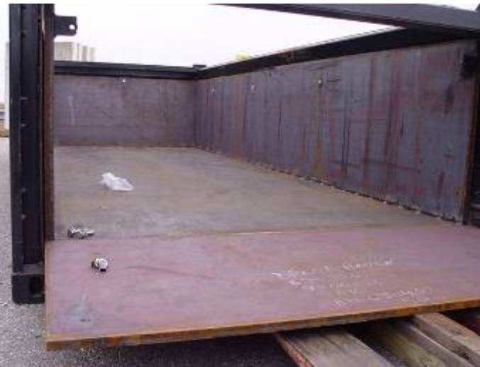
One of the five intermodal containers which had shielding designed and installed by BSA engineers and technicians. These containers were modified specifically to transport the highly-activated neutron shields.
