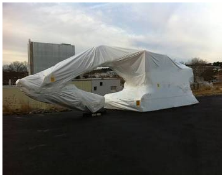
New Holland excavator in "supersack" ready for transfer to another DOE project at Paducah, KY.
