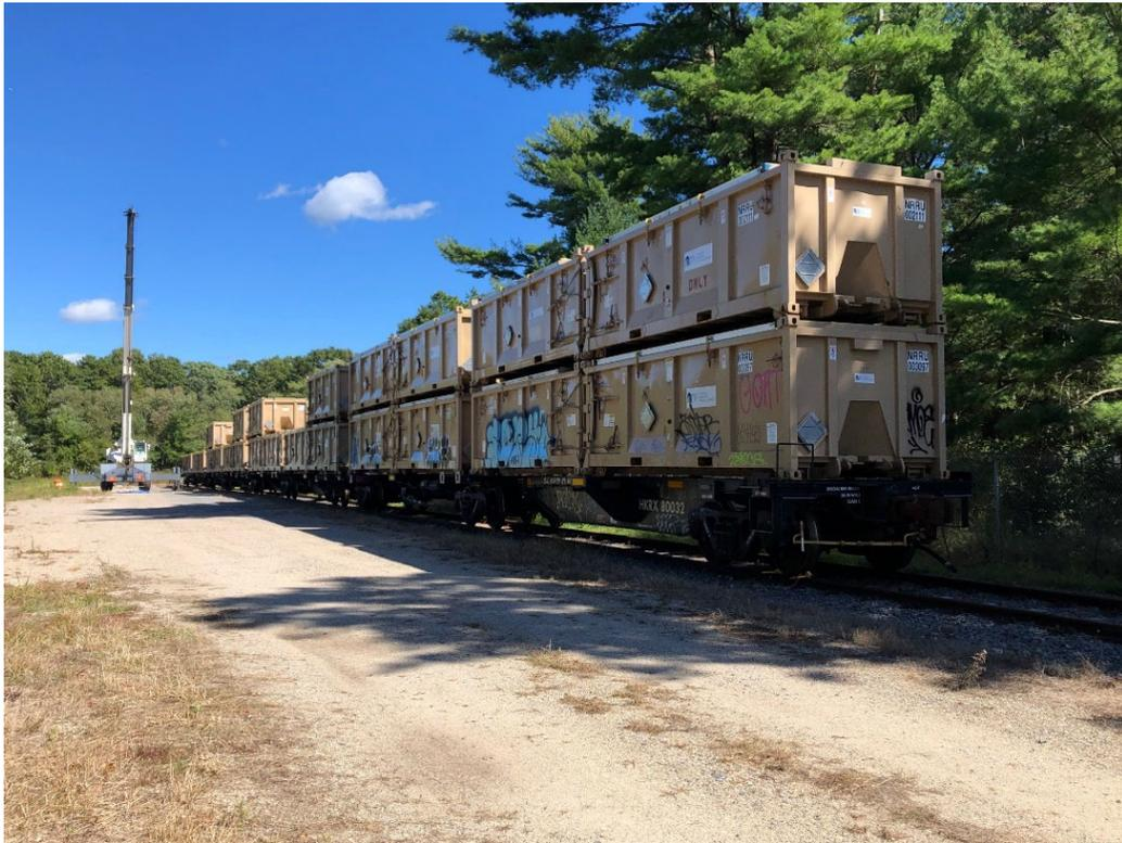
**Photograph 7 – Intermodals Loaded on Railcars for Offsite Disposal**
