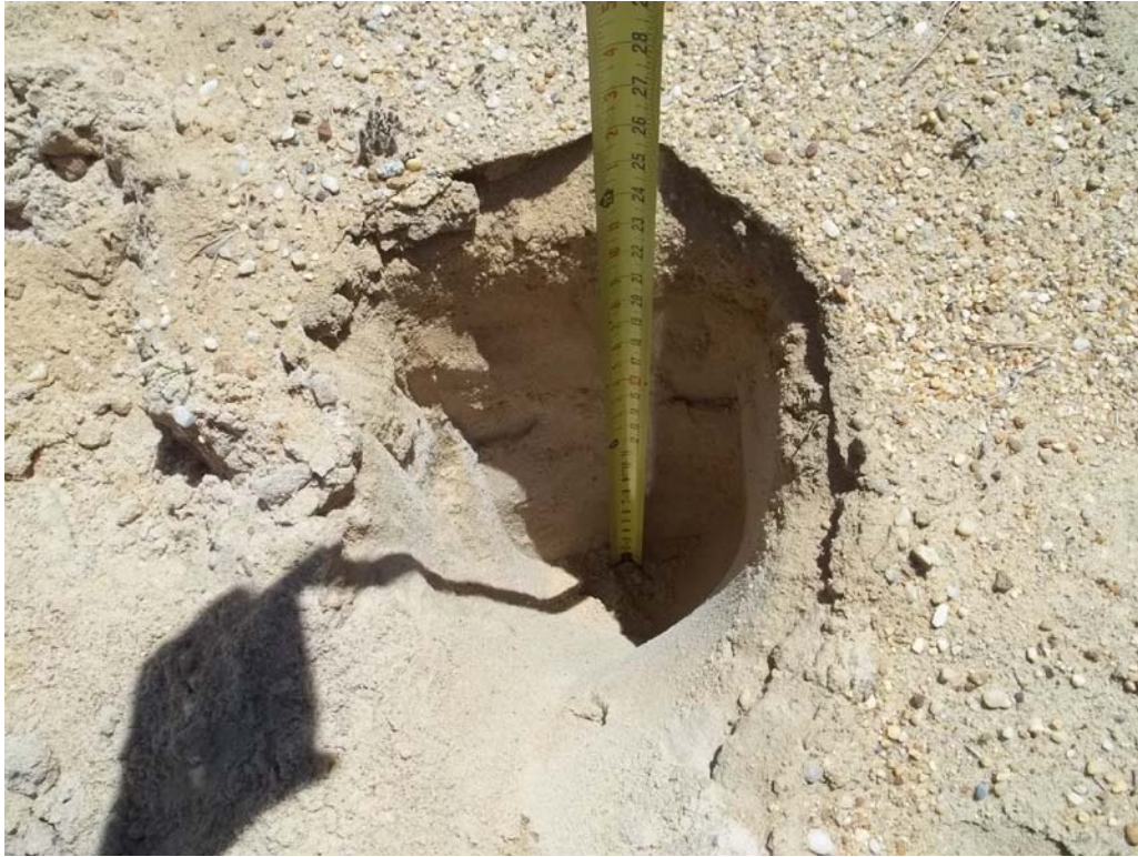
Photograph 5: Minimum 18-inch soil cover at landfill area.
