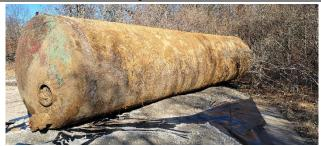
Photo 3-33x8ft single steel wall UST looking at the eastern end cap and northern sidewall. No pitting or holes were observed.
