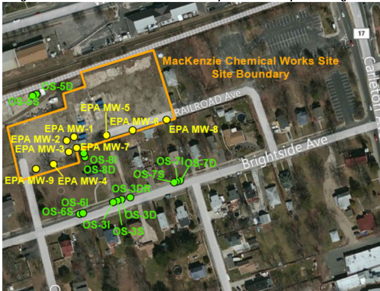
Figure 1: MacKenzie Chemical Works – Site Layout with Nearby Monitoring Wells
