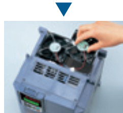
Disconnect the power connector and change the cooling fan cartridge.
