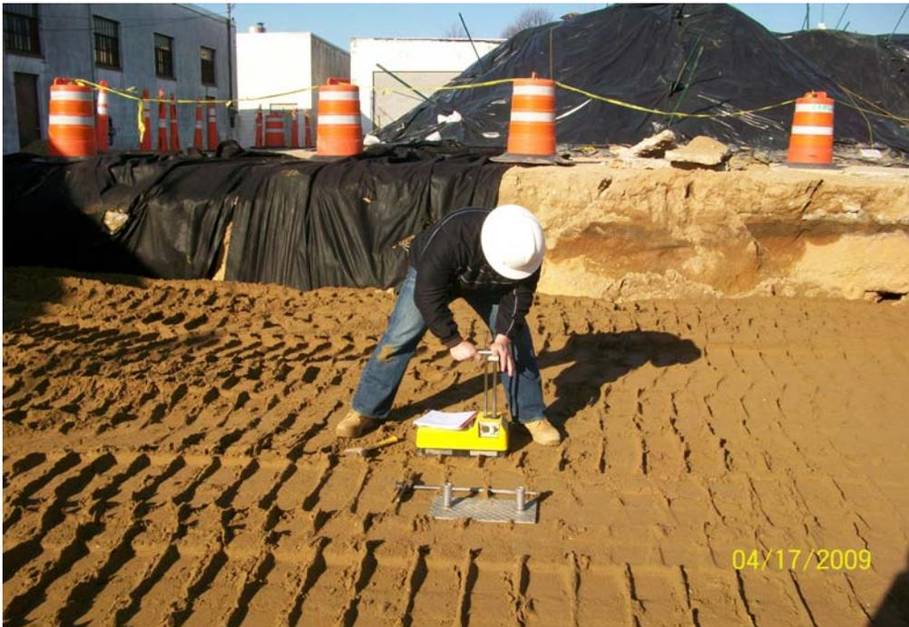
100\_00377.jpg - Soil Mechanics technician collecting compaction test data.
