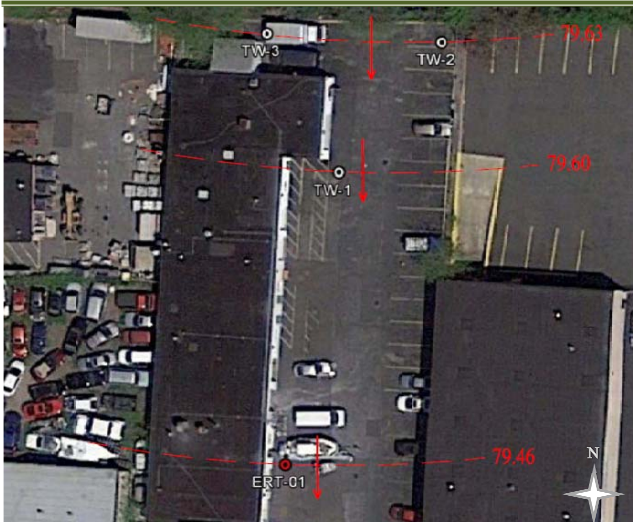
Figure 4: Groundwater Elevation/Flow Direction Map – September 2016
