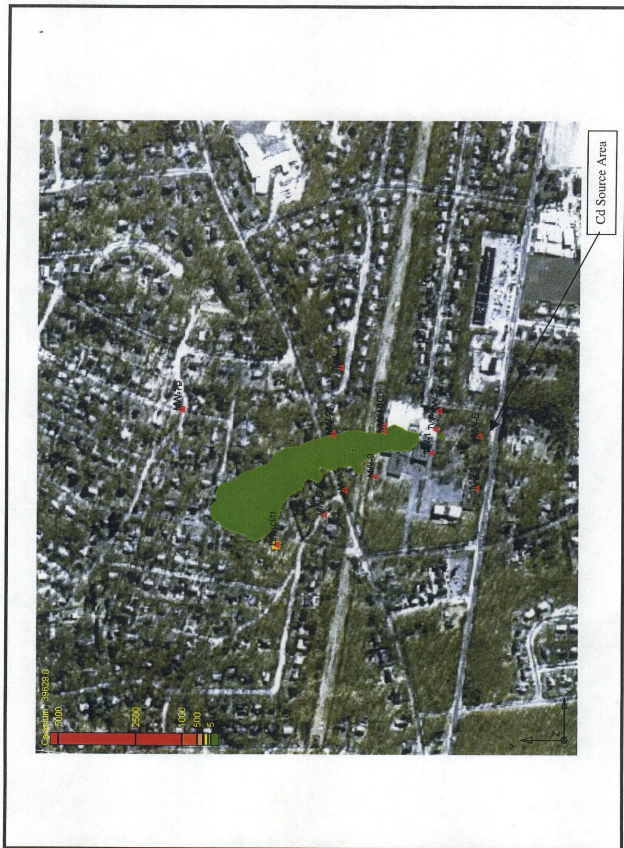
Figure A.2-18. Graphic representation of predicted cadmium concentrations for model Layer 3 (31 January 2103).
