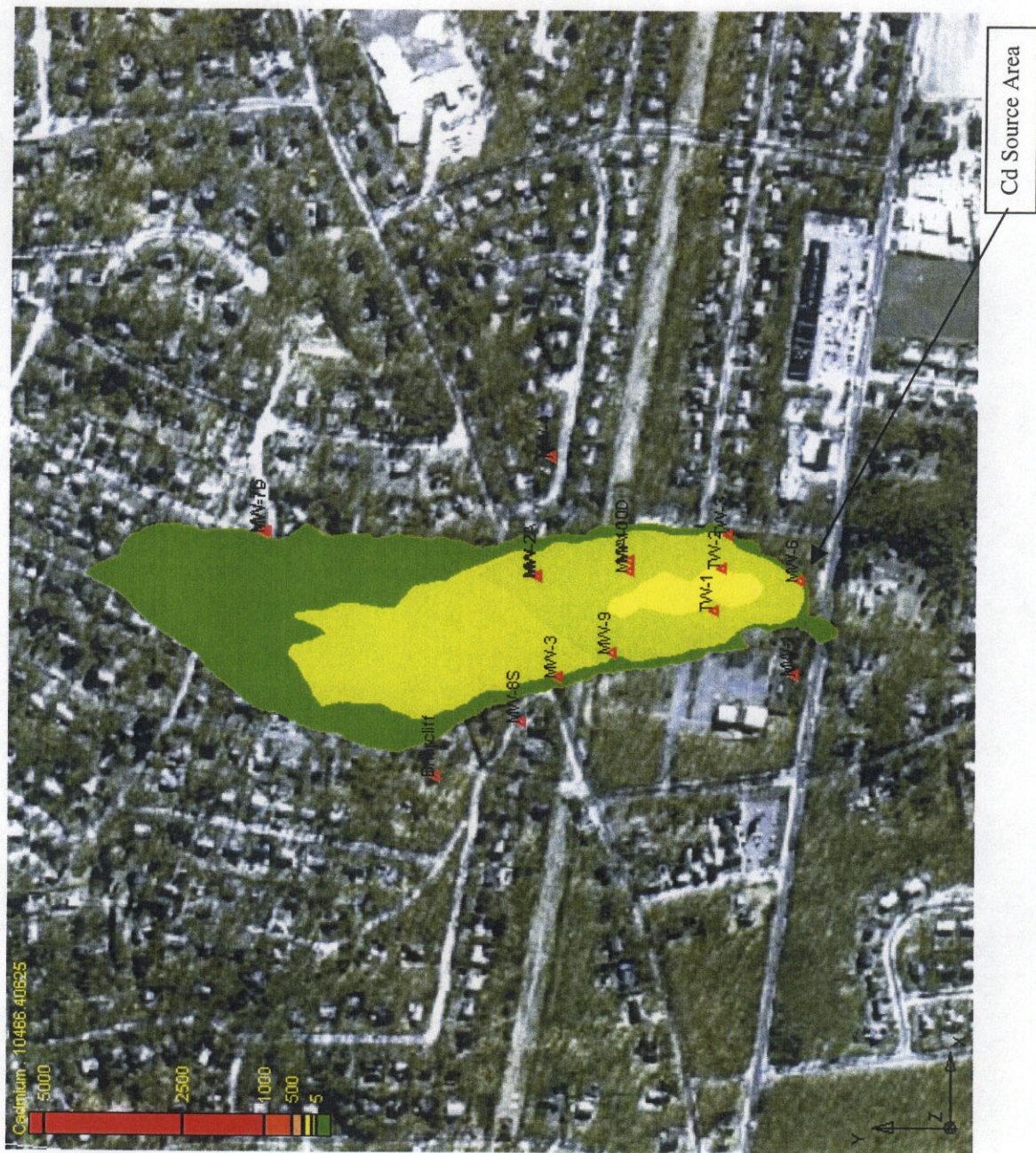
Figure A.2-9. Graphic representation of predicted cadmium concentrations for model Layer 2 (5 March 2023).
