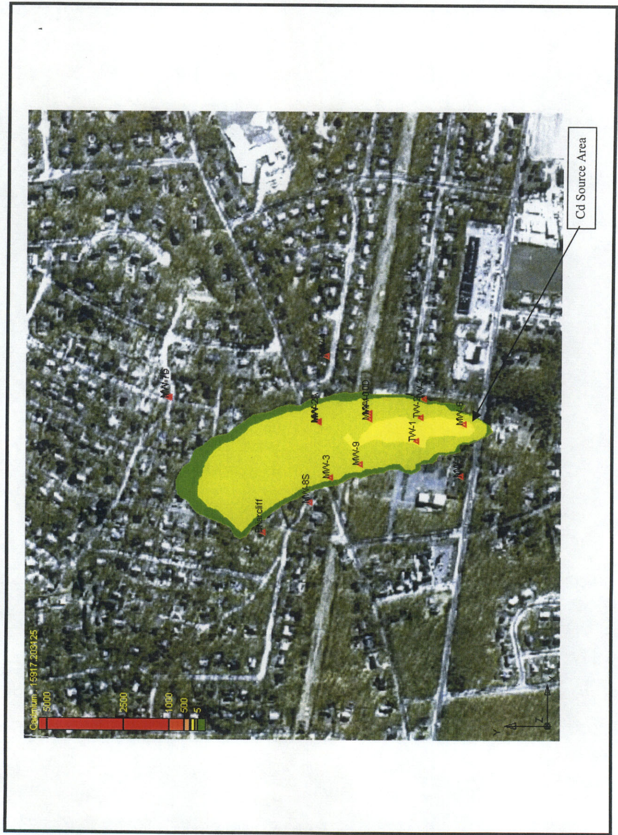
Figure A.2-10. Graphic representation of predicted cadmium concentrations for model Layer 2 (17 February 2038).
