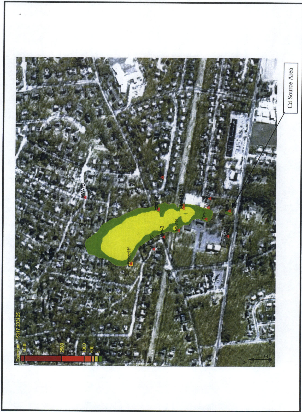
Figure A.3-16. Graphic representation of predicted cadmium concentrations for model Layer 3 (17 February 2038).
