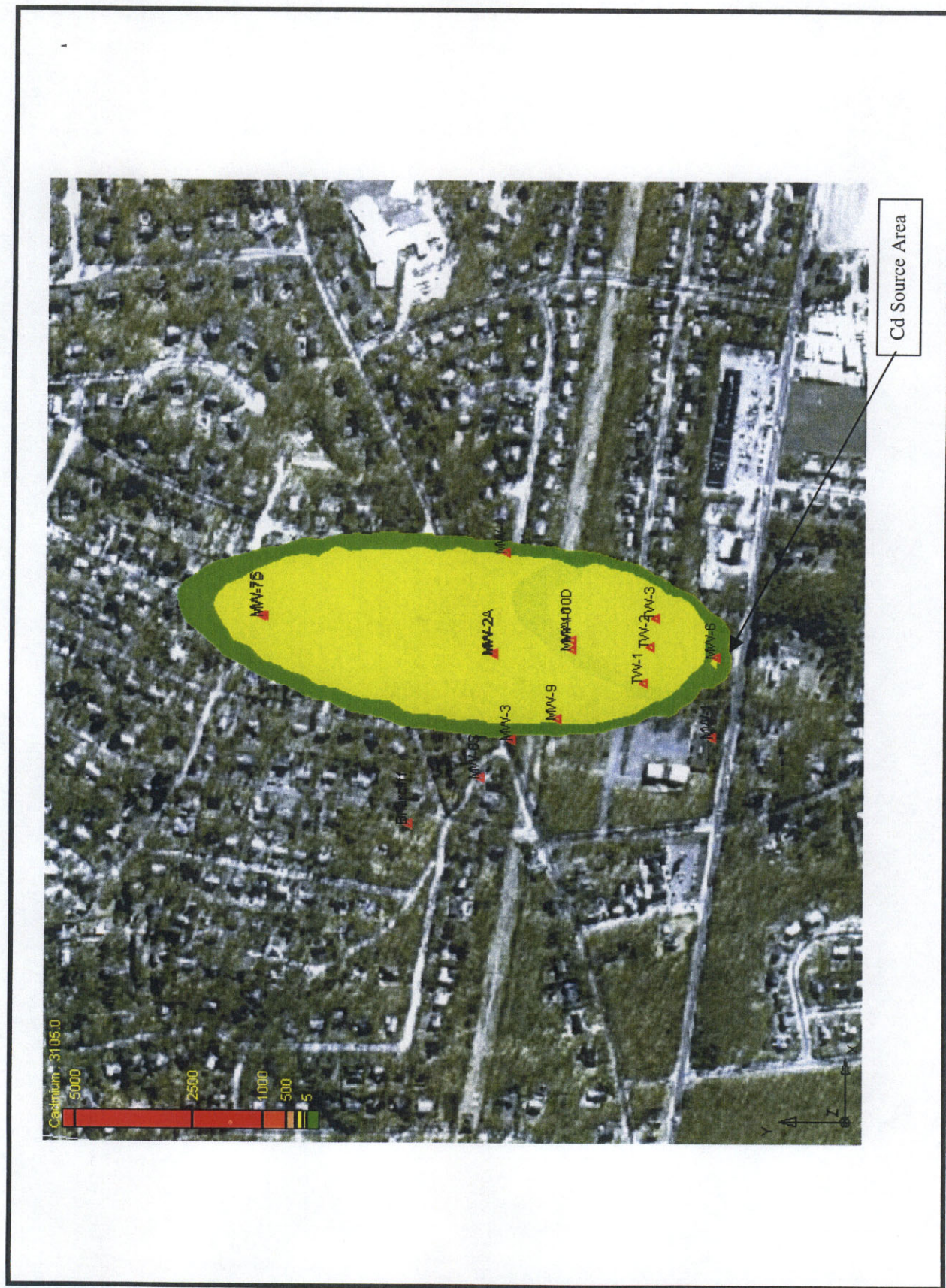
Figure A.2-7. Graphic representation of predicted cadmium concentrations for model Layer 2 (31 January 2003).
