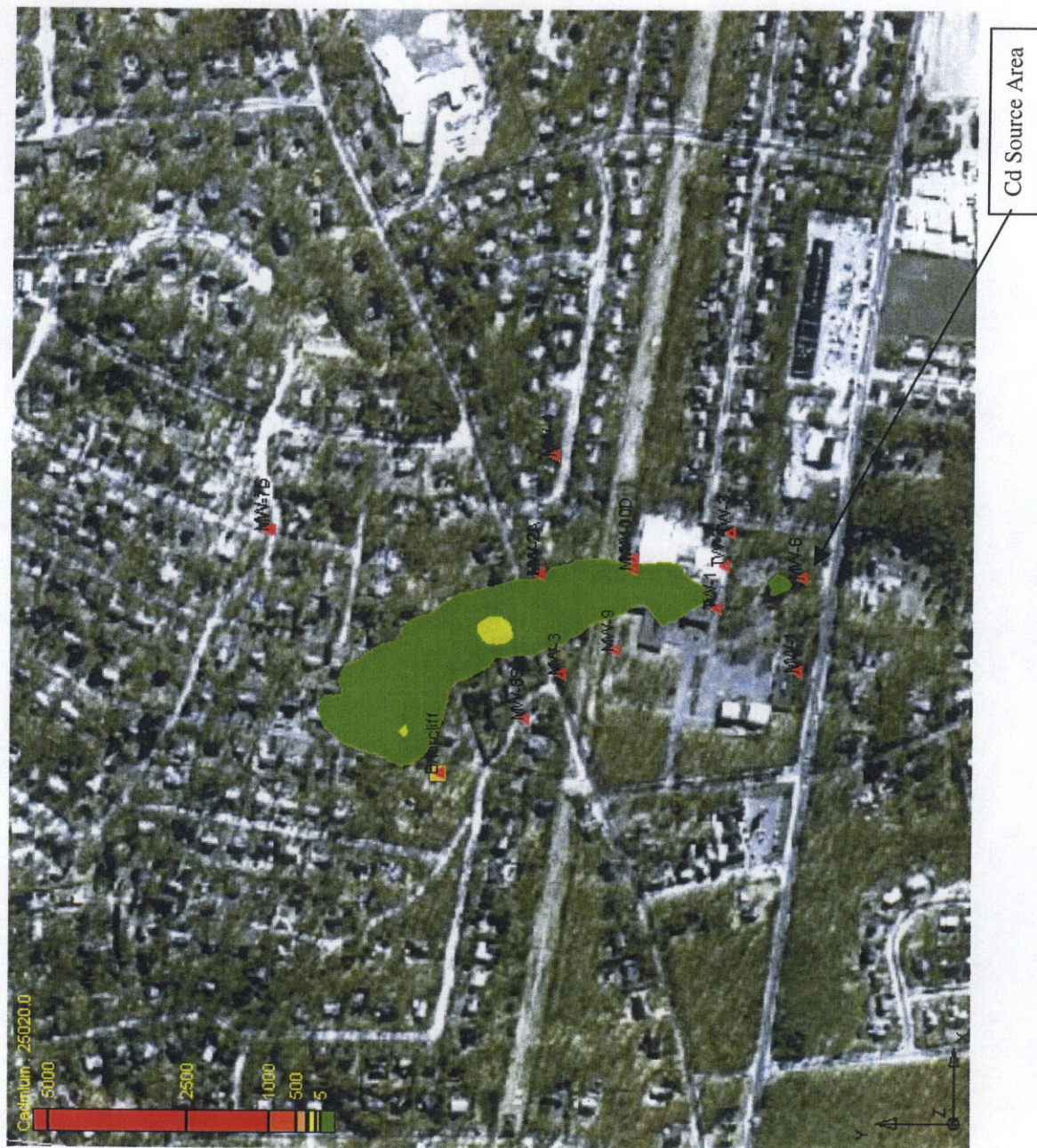
Figure A.2-17. Graphic representation of predicted cadmium concentrations for model Layer 3 (31 January 2063).
