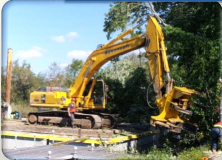
Tree Shear attachment and equipment used to remove trees around Lake Capri
