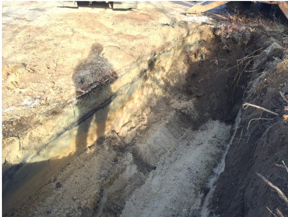
SB-18, discovery of petroleum-like impacted soils from 0.5' to 2'.
