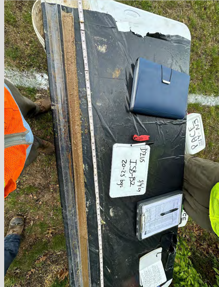
20-25' bgs section of soil boring at ISB-B2 boring location.
