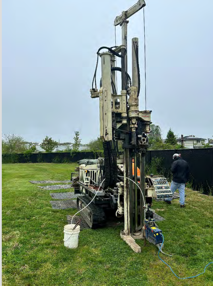
SP16 in-situ groundwater sampling set up on Geoprobe rig.
