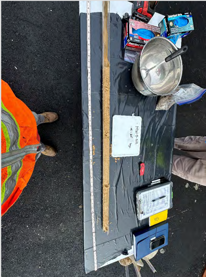
MW-9-SB soil core from 15-20' bgs. Soil sample collected from the 19-20' bgs interval.
