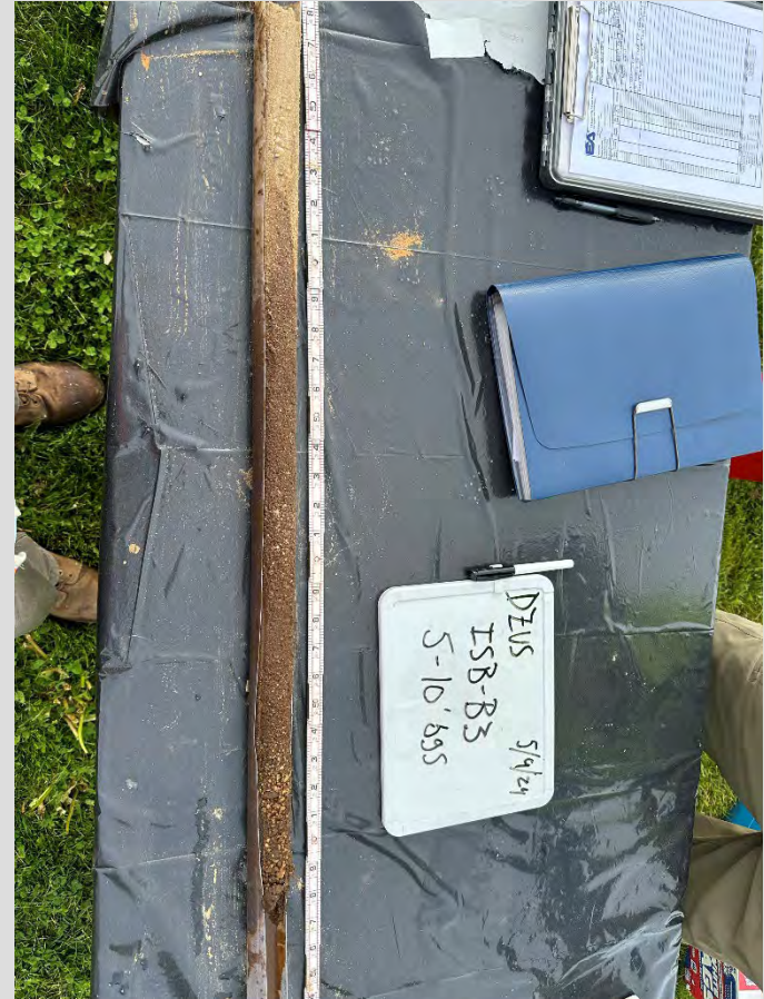
5-10' bgs section of soil boring at ISB-B3 location.
