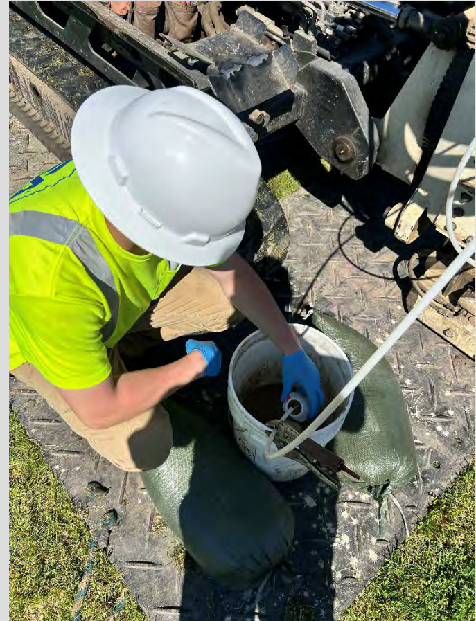
EA collecting unfiltered in-situ groundwater grab sample at sampling location ISB-D3.
