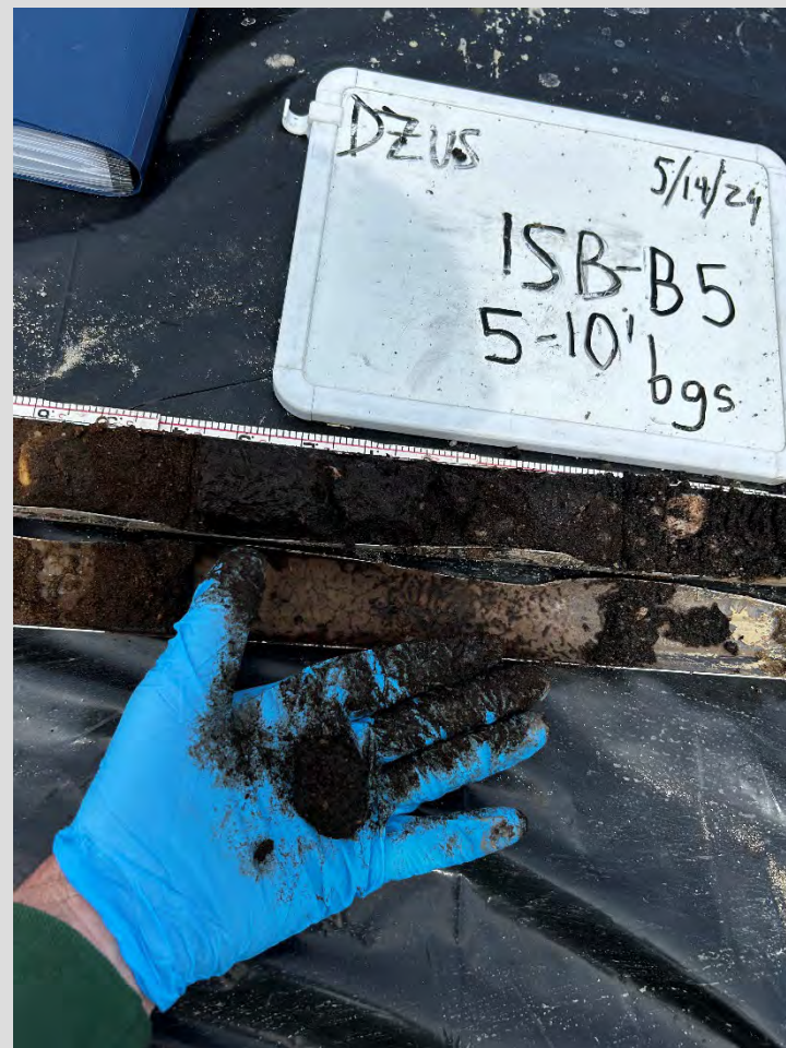
ISB-B5 7-8' bgs, saturated organic peat-like Material.
