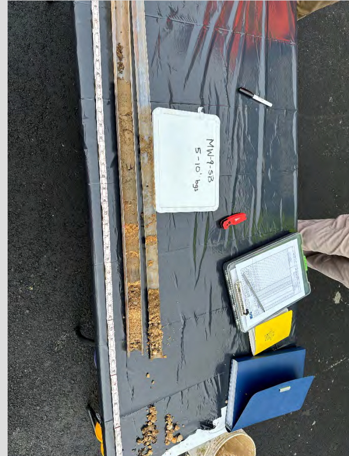
MW-9-SB soil core from 5-10' bgs. Soil sample collected from this interval.
