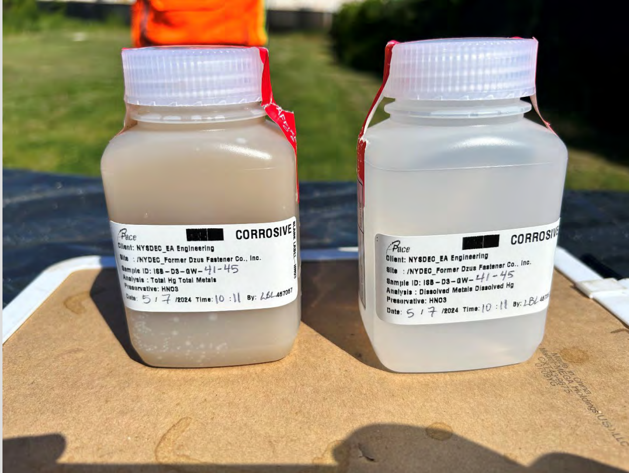
Unfiltered (left) and filtered (right) groundwater samples from ISB-D3 sampling location.
