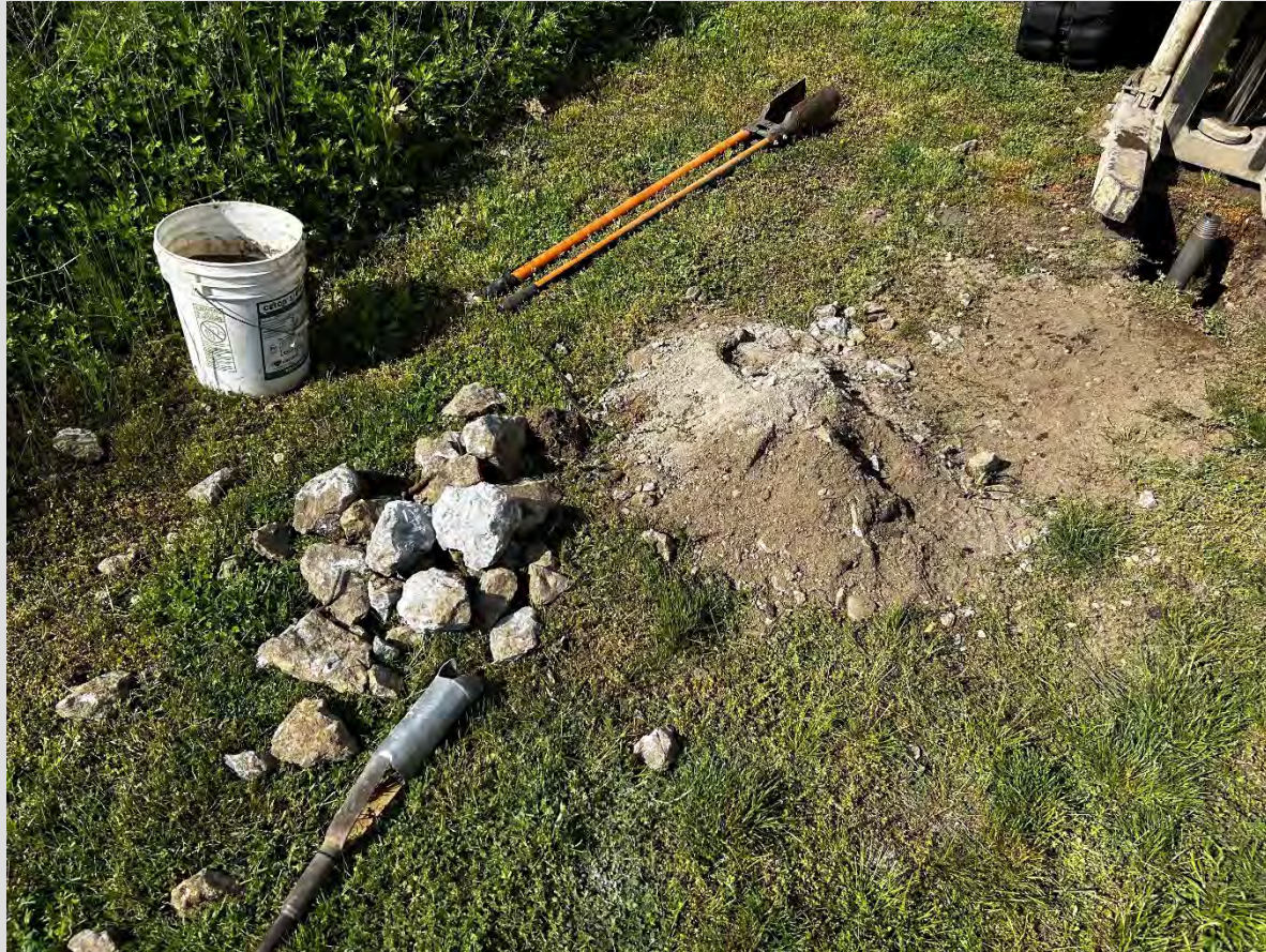
Large rip rap pile and sandy silt from top 5' of ISB-B4 boring.
